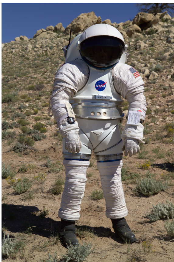
Figure 1-1: Picture of the Mark III suit. Above the waist is the Hard Upper Torso (HUT), below the waist is the Hip Bearing Assembly (HBA). Source: NASA [22].
