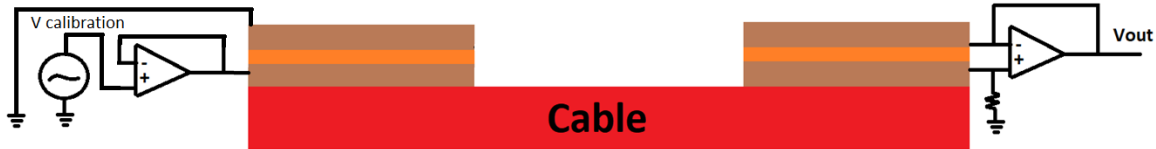
Figure 5-13: To calibrate the system, we apply a known signal to the calibrating electrode, represented on the left side of the figure, which capacitively injects a voltage into the cable that then creates a voltage in the sensing electrode.
