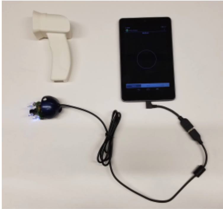
Figure 4-1: The device used to capture iris images alongside hood attachment [2]
