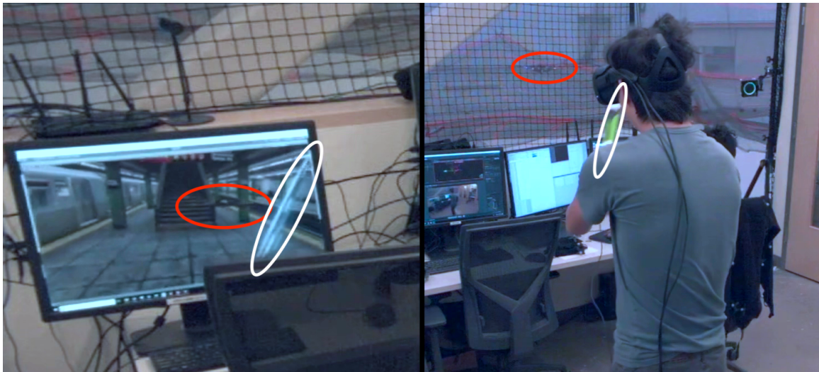
Figure 4-25: Dynamic actor using VR to interact with a drone in flight using a virtual prop held by the actor. The drone in flight is circled in red, the dynamic prop held by the actor is circled in white.
