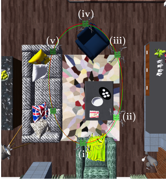
(a) Trajectory from a single oval of VIO-in-the-loop flight overlaid on the environment 3D model. The green line shows the position of the drone as recorded from motion capture while the red line shows the VIO state estimate of position used for control.
