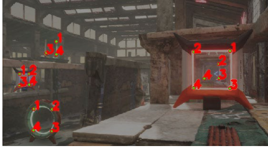
Figure 3-3: Rendered camera view (faded) with IR marker locations overlaid. The unprocessed measurements and marker IDs from the simulated IR beacon sensor are indicated in red. The measurements are verified by comparison to image-space projections of ground-truth IR marker locations, which are indicated in green. Note that IR markers can be arbitrarily placed by the user, including on dynamic objects.
