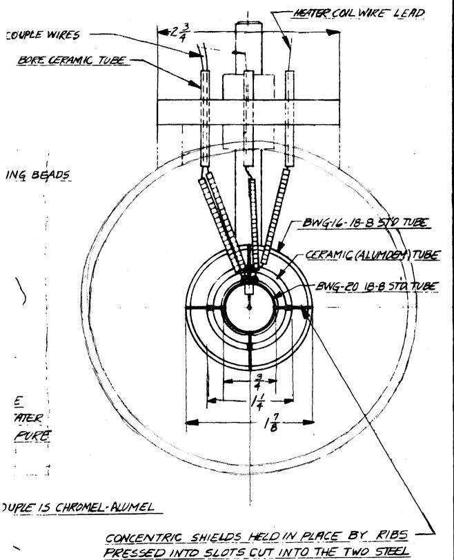
CONCENTRIC SHIELDS HELD IN PLACE BY RIBS PRESSED INTO SLOTS CUT INTO THE TWO STEEL
