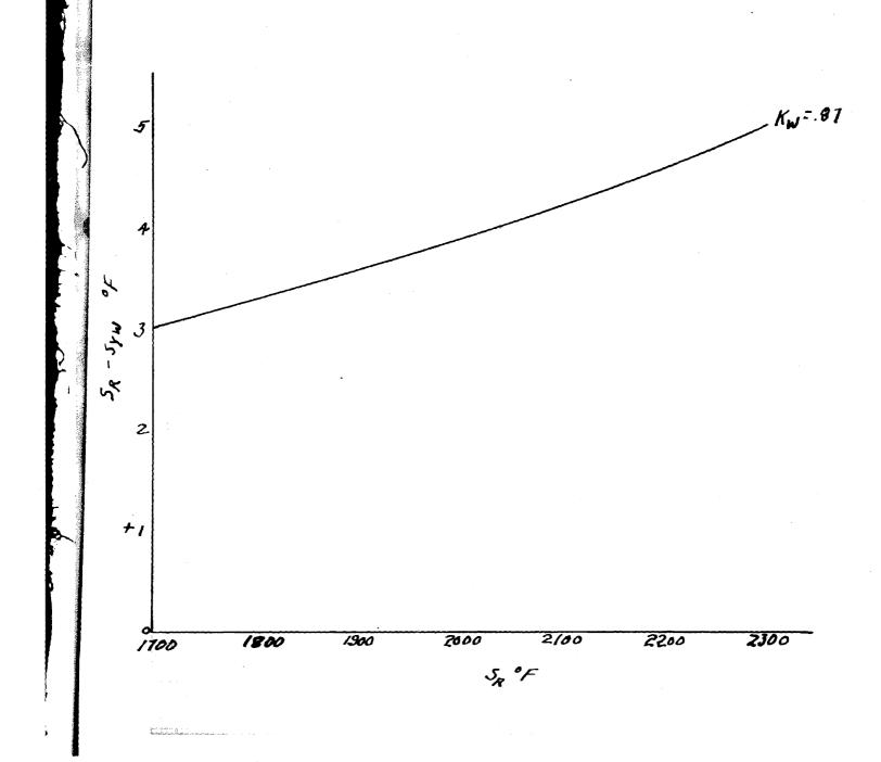
Plot of Sodium Line Reversal Measurements is. Thermocouple Readings for Two Runs
