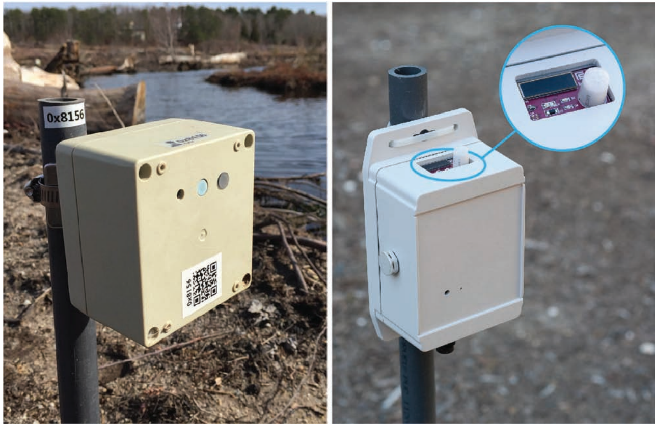
Figure 5. Left: first-generation sensor node in its enclosure, installed in the field. Right: second-generation sensor node prototype, with inset showing optical components on top of the node (detailed in Figure 4).
