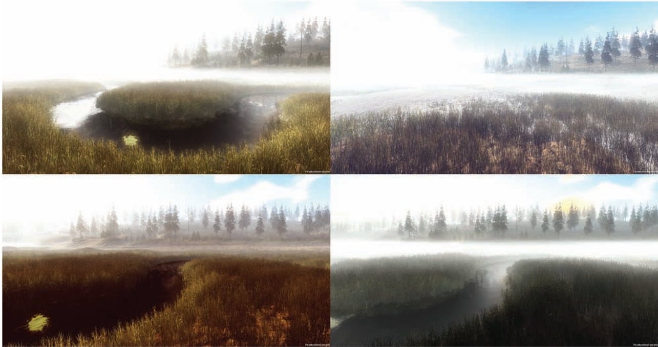
Figure 14. Doppelmarsch virtual weather patterns: fog is controlled by nearby humidity sensors, and rain intensity by precipitation meters. Sensor data are combined with machine vision on the camera images to control rendering of snowpack and vegetation.
