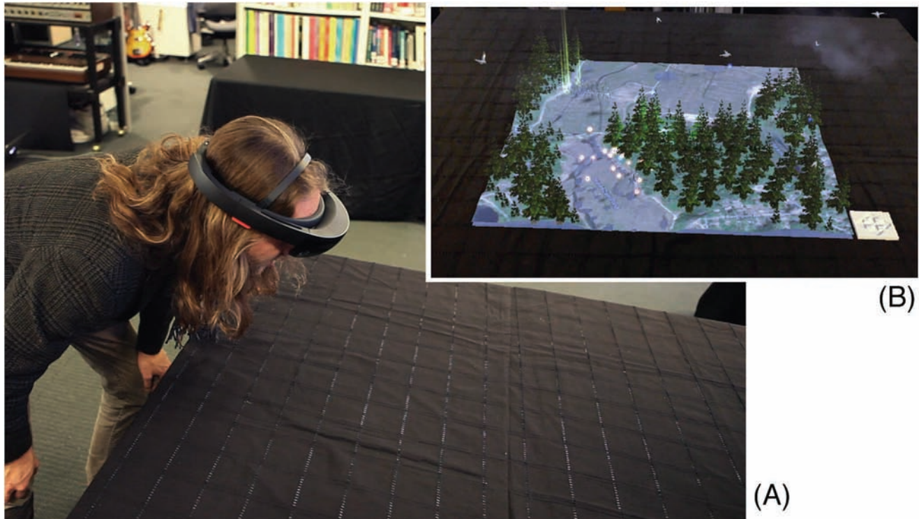
Figure 16. Hakoniwa uses a head-mounted augmented reality display (A) to render a real-time sensor-driven miniature marsh landscape on a tabletop (B).
