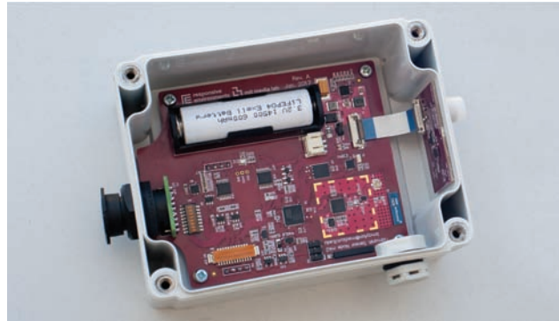
Figure 3. The second-generation hardware inside the waterproof enclosure.
