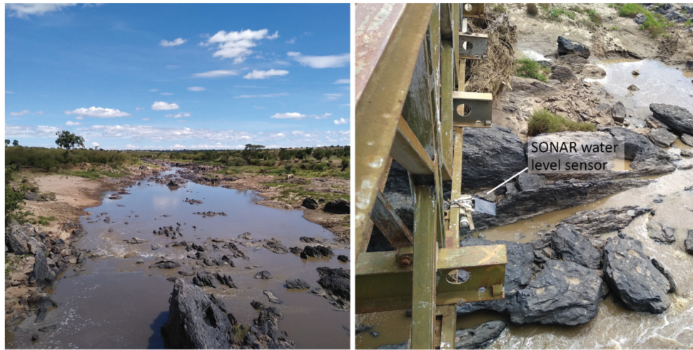
Figure 9. The Mara River in the Maasai Mara National Reserve ( left ), and a SONAR level sensor installed on a bridge over the Mara River ( right ).
