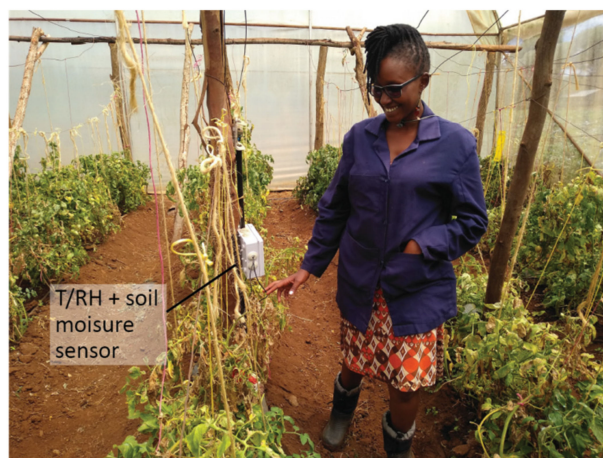
Figure 10. Greenhouse Supervisor inspecting tomatoes and a temperature, humidity, and soil moisture device in a greenhouse at the Dedan Kimathi University of Technology research farm.
