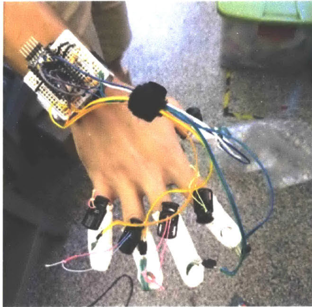
Figure 3-3: Force Sensing Resistors mounted to each of the person's fingertips.
