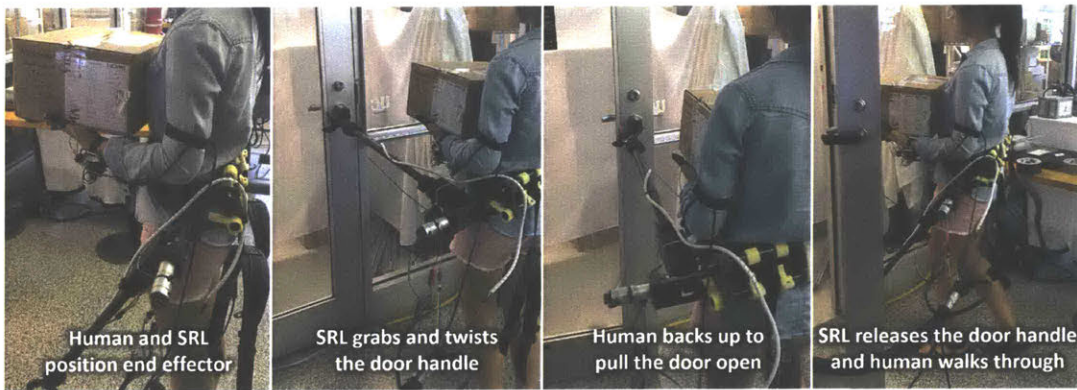
Figure 3-7: Demonstration of the Superlimb. In the first image, the human operator and Superlimb work together to position the end effector in x, y, and z. In the second image, the human operator commands the Superlimb to grab and twist the door handle with a single code. In the third image, the human operator backs up to open the door. Finally, in the last image the human operator commands the Superlimb to release the door handle. The human operator is then free to walk through the door.
