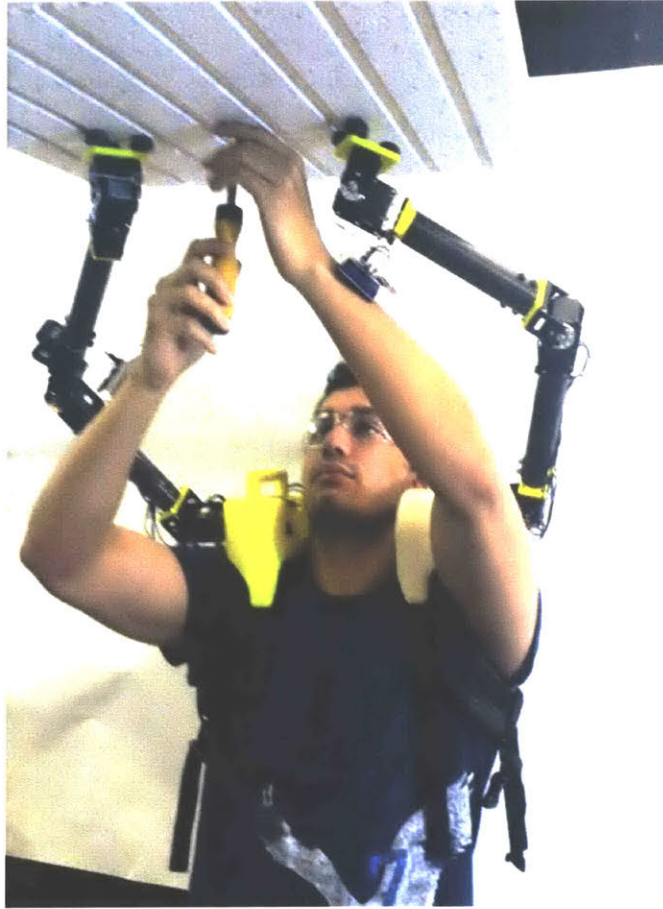
Figure 4-1: A pair of Superlimbs sitting on the shoulder of a human operator. The human operator feels the reaction force from the Superlimbs holding the ceiling panel in place.
