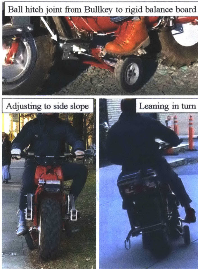
Figure 4-5: The balance is a rigid, wheeled platform connected to the motorcycle frame by a ball hitch. The user steps on the balance board to stabilize themselves but can still comfortably stay upright on side slopes or lean in turns.
