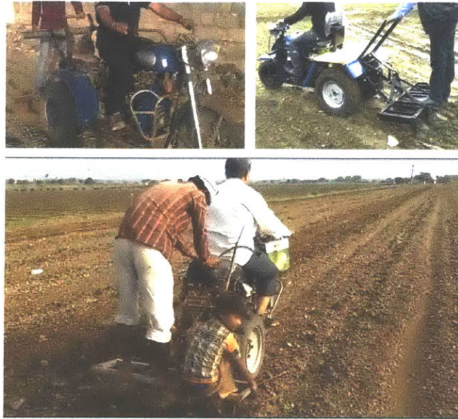
Figure 5-1: Images of people riding on tools to help them sink into the ground. These are tools mounted on conventional three point hitch linkages but that are manually operated.
