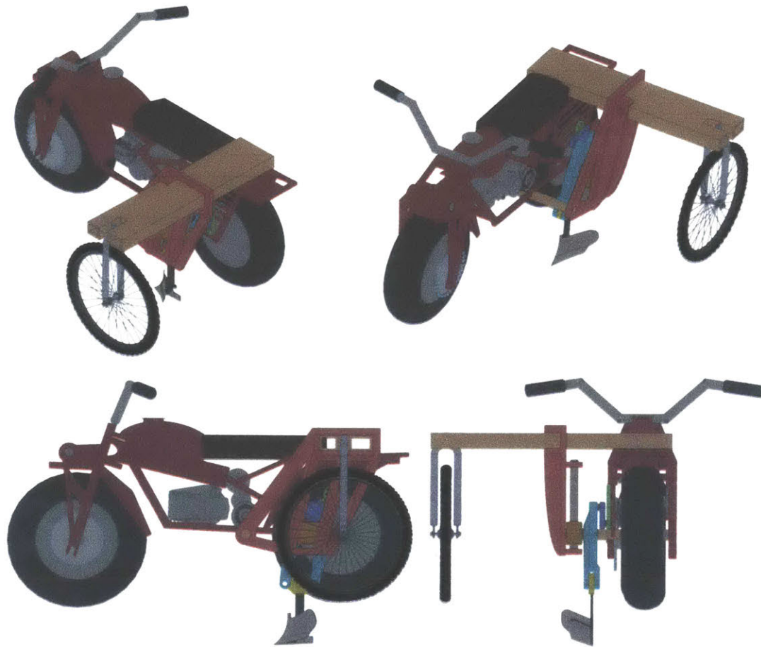
Figure 6-11: Views of concept sliding rail mechanism on motorcycle.
