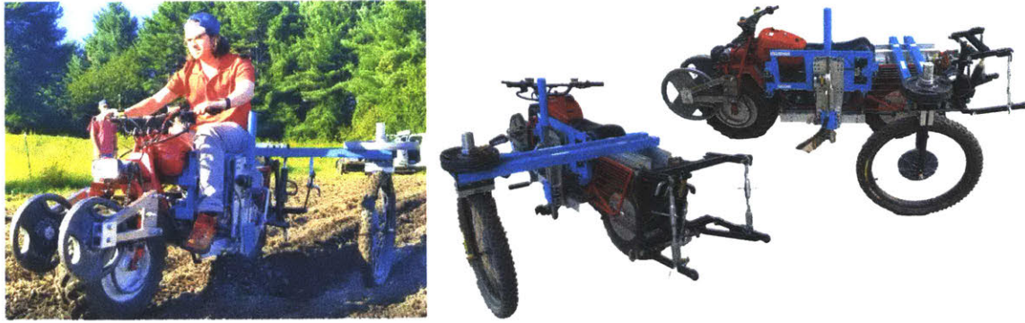
Figure 1-1: Images of the proposed Bullkey tractor. This design is discussed in detail in Chapters 3 and 4. It features inline drive wheels, an outrigger wheel, and an option for a centrally located tillage tool or conventional rear mounted tools.
