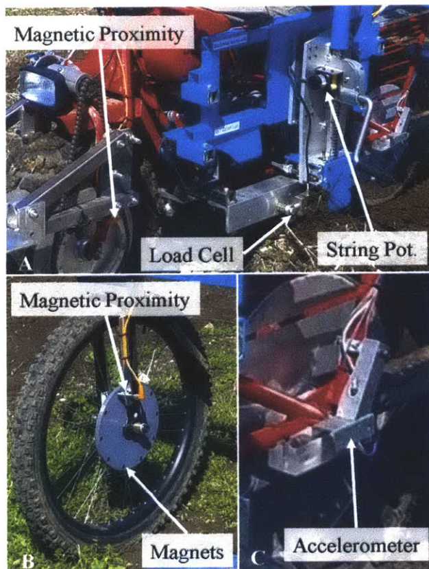
Figure 3-11: Close-up views of sensor installation examples. Views of prototype shown are (A) left-side, (B) outrigger wheel right side, and (C) rear axle left side
