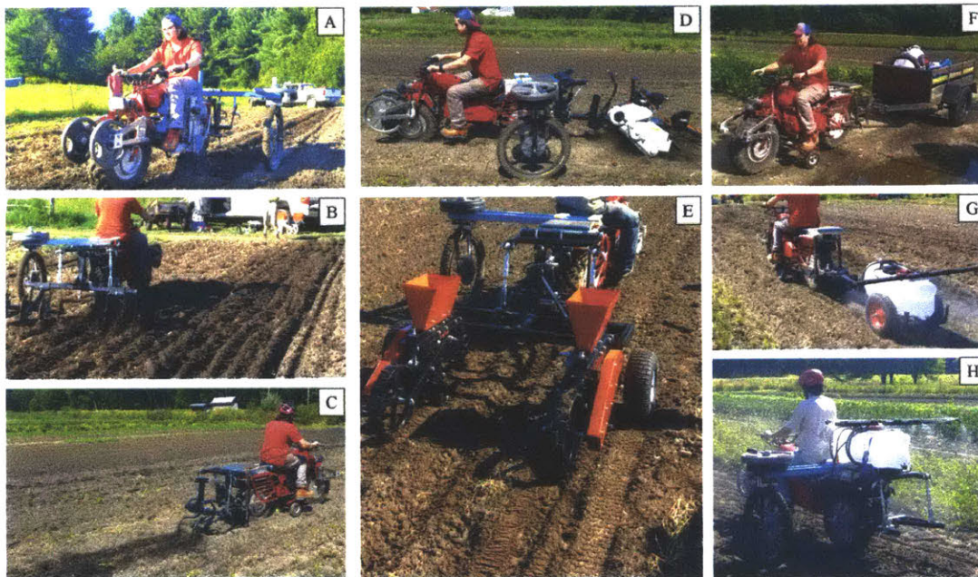
Figure 4-8: Images of the researchers performing key operations of interest to Indian farmers with Bullkey. A) Plow B) Disc harrows C) Cultivator D) Rotavator E) Planter F) Trailer G) Sprayer on its trailer H) Sprayer on motorcycle.
