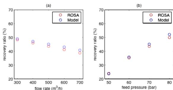
Figure 7. RO model verification: (a) varying feed flow rate; (b) varying feed pressure
