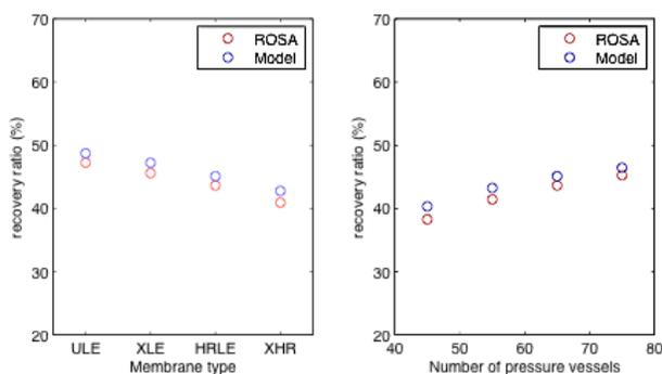
Figure 8. RO model verification: (a) different types of RO membrane element; (b) varying number
