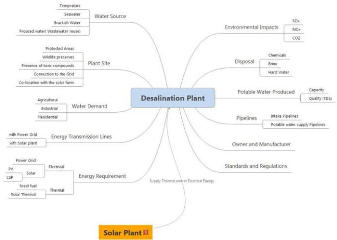
Figure 2. Desalination plant as a black box with its external dependencies and linkage to the solar plant
