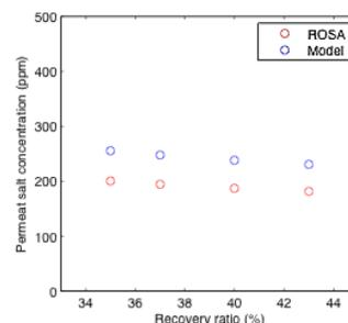
Figure 9. RO model verification, salt concentration, and recovery ratio
