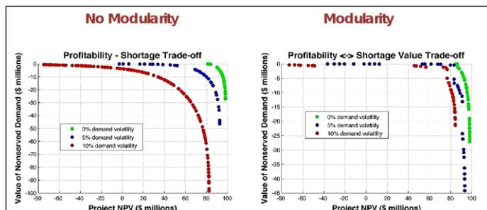
Figure 5. Pareto trade-offs in monolithic/non-modular (left) and modular (right) plant designs, with modular presenting knee points that simultaneously maximize project NPV and minimize the social losses of unserved demand
