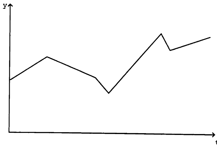
Figure 2.6: Particle moving with piecewise constant velocity. The length of each segment is exponentially distributed.
