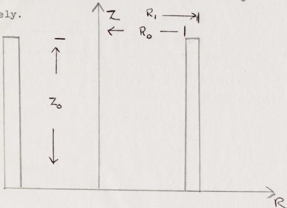
Let  $T_A$  be the ambient temperature which is assumed to be constant. Also we will assume the bottom of the cup is very well insulated and that heat loss is negligible. Constructing a heat balance on a differential volume element of the substance to be maintained will yield the following equation.
