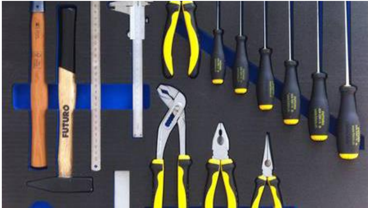
Figure 7-3: Example of tool shadow-kitting. Source: osaapamerica.com/products/kitting
