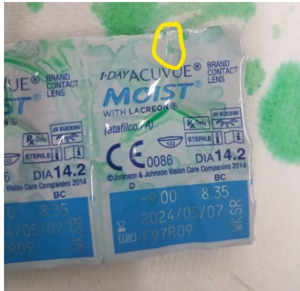
Figure 5-6: Heat seal failure example from a controlled experiment
