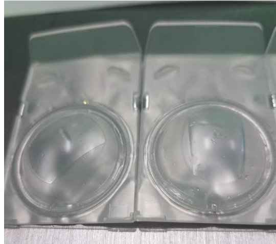
Figure 5-3: Example of a contact lens folded in on itself (sample was collected in a controlled experiment)
