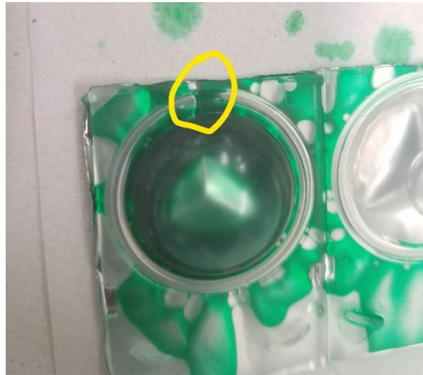
Figure 5-5: Heat seal failure example from a controlled experiment
