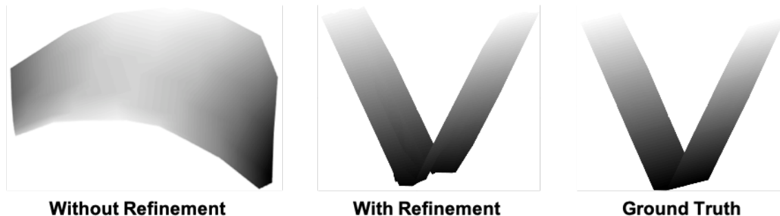
Figure 4-5: Comparing Reconstructed Shape: Using RANSAC to refine our point partition preserves the underlying shape.
