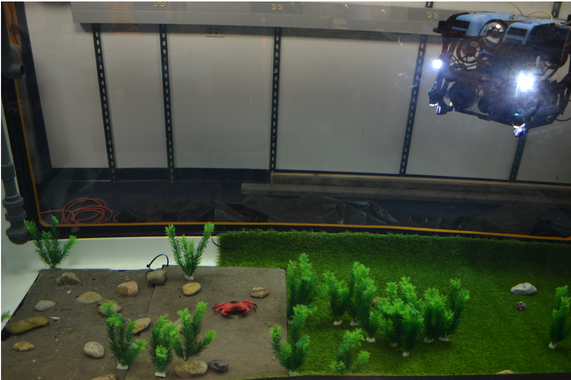
Figure A-3: Here we show the WARPLab AUV “Red”, a modified BlueRobotics BlueROV, exploring an artificially created underwater environment at WHOI. Appeared in [42].
