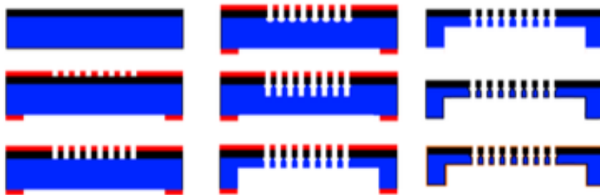
Figure 38: Cross sectional overview of electrowetting valve fabrication flow. [14]
