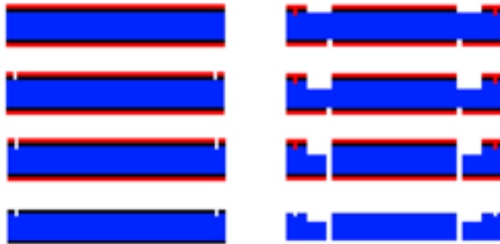
Figure 33: L3 alignment layer cross-section evolution. There are notched steps to both hold the shallow etched alignment crosses and support the extractor. [14]
