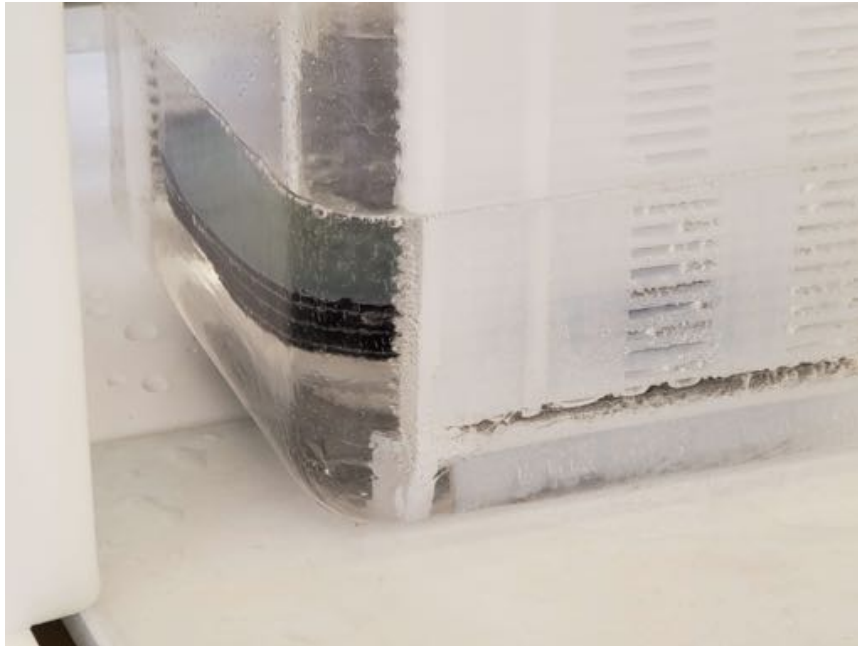
Figure 35: Piranha solution stripping photoresist and organic materials from wafers prior to bonding.
