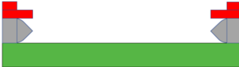
Figure 5: Frame cross section. Green is the silicon base layer "L1," Gray is the glass insulating layer "L2" with a knife edge to retain liquid, and red is the silicon alignment layer "L3."
