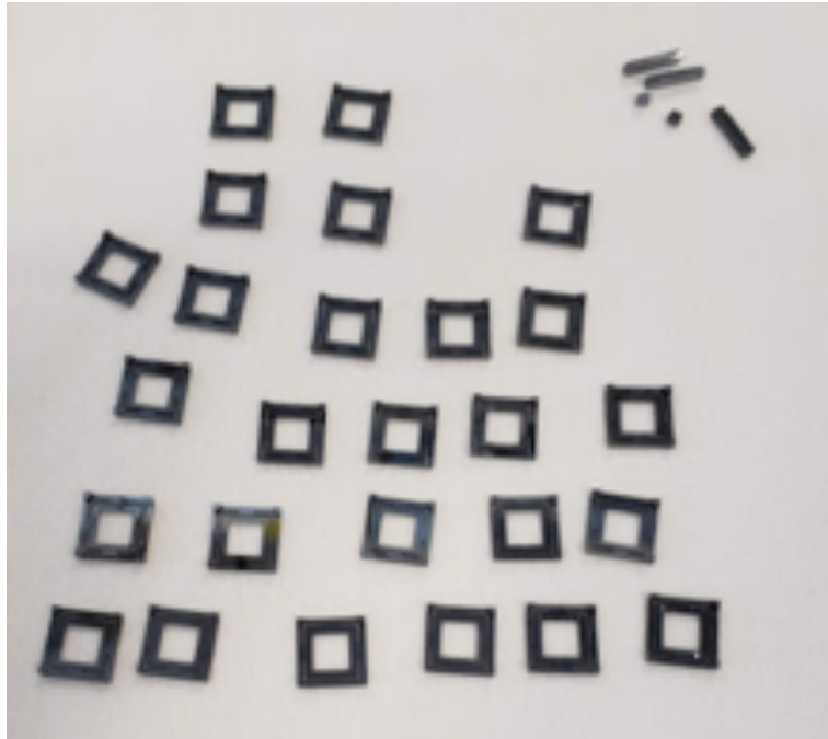
Figure 37: Frames after dicing and acetone bath.
