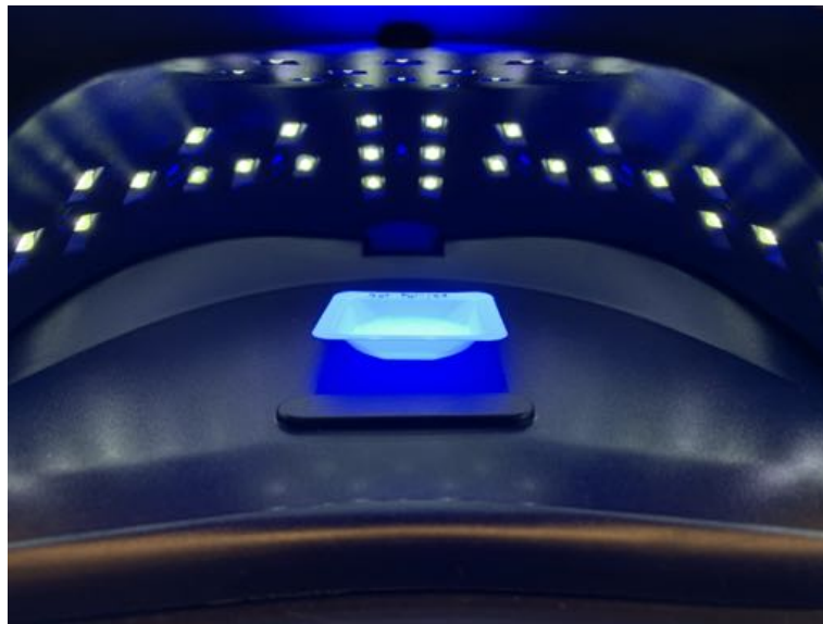
Figure 51: First trial of commercial UV source on a resin batch in an open-top teflon dish.
