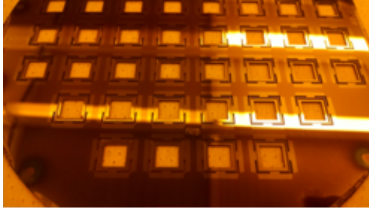
Figure 11: A revised L1 wafer. The well and moat features are clearly visible; the diffraction pattern at the edges of the wafer is produced by the clamps that hold the wafer to the chuck in the DRIE tool and have no effect on the functionality. [14]
