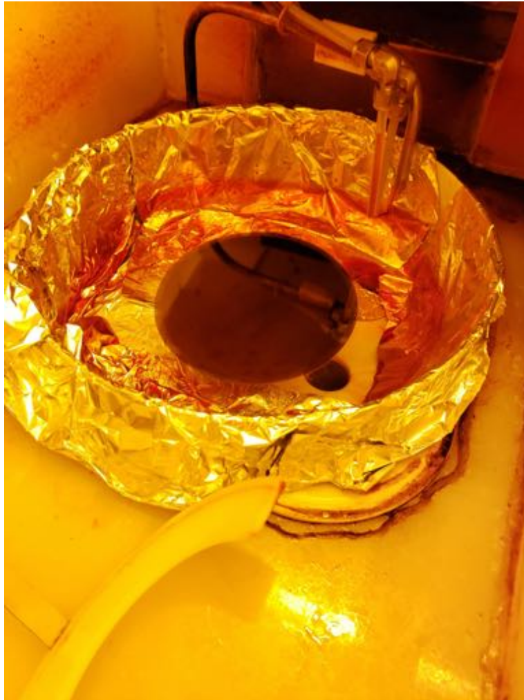
Figure 25: Spin coating a wafer with AZ4620 “thick” photoresist. Note the aluminum foil is used only to make resist cleanup easier.
