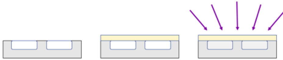
Figure 50: UV curing of the resin mix into solid chips. From left to right, the PDMS mold (gray) is filled with uncured resin (white), a glass slide (yellow) is used to keep the curing chips from warping, the UV source (purple) is activated and the chips are cured for 10 minutes.
