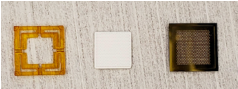
Figure 12: iEPS v3 SLA printed frames made of Cyanate Ester (left) shown with emitter chip (center) and extractor (right).
