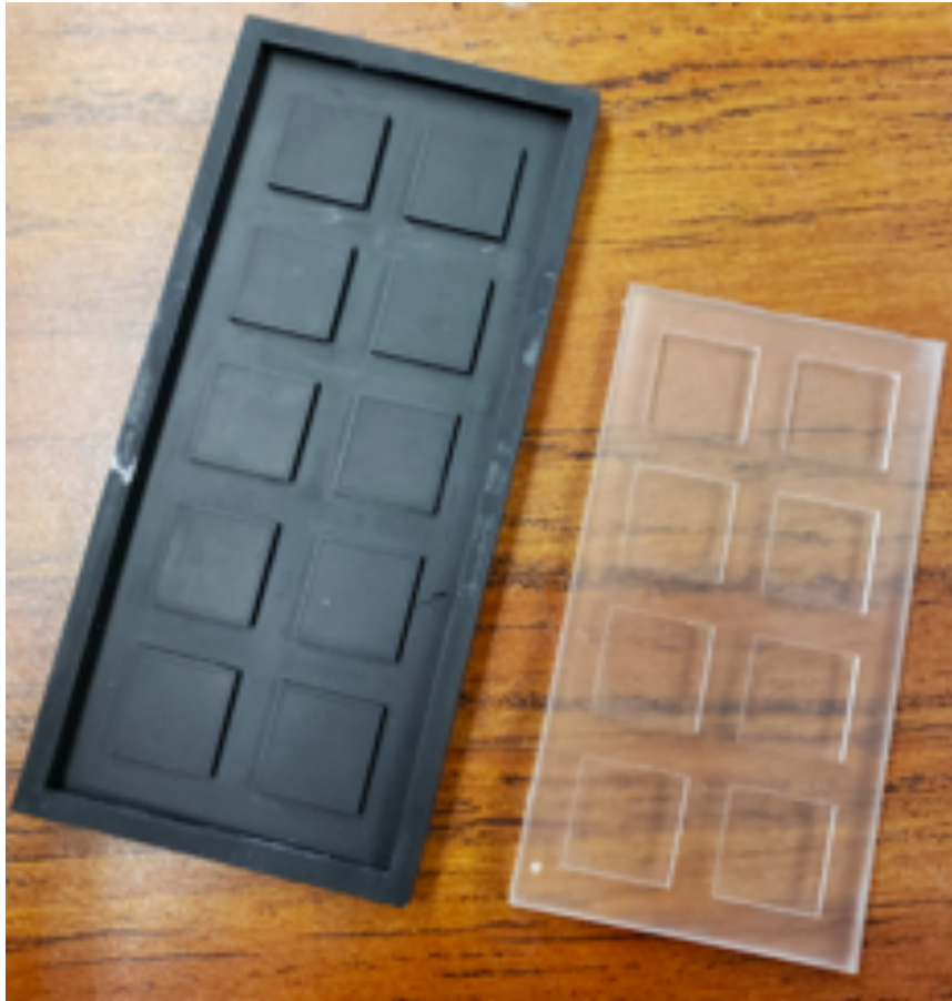
Figure 49: ABS and PDMS positive and negative molds used for casting the silica/resin suspension into chips.
