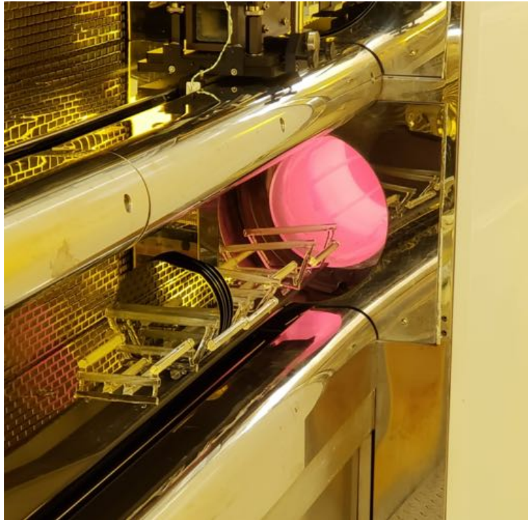
Figure 24: Wafers entering a furnace for thermal oxide growth. The quartz holder is needed to withstand the hot environment.
