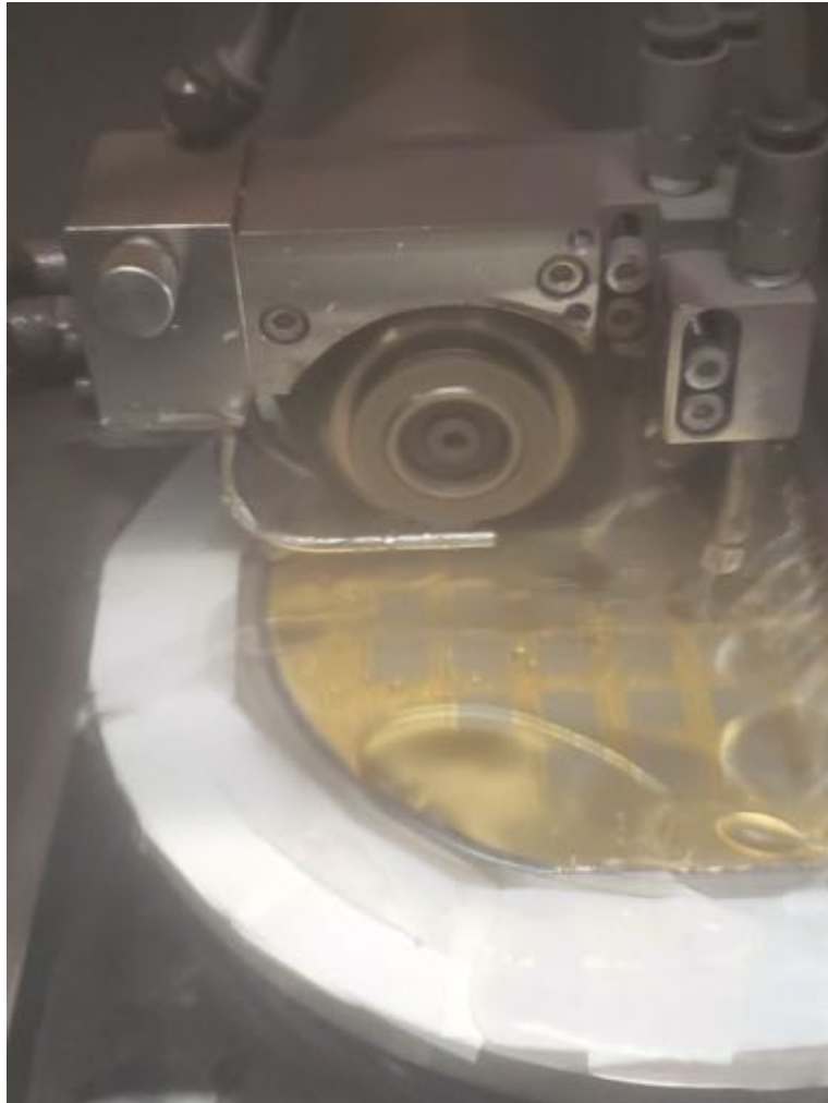
Figure 28: Dicing a developmental extractor wafer. The wafer is mounted on dicing tape, which in turn is attached to the chuck via vacuum. The white tape around the edge is intended to prevent water getting underneath the tape and potentially lifting it.
