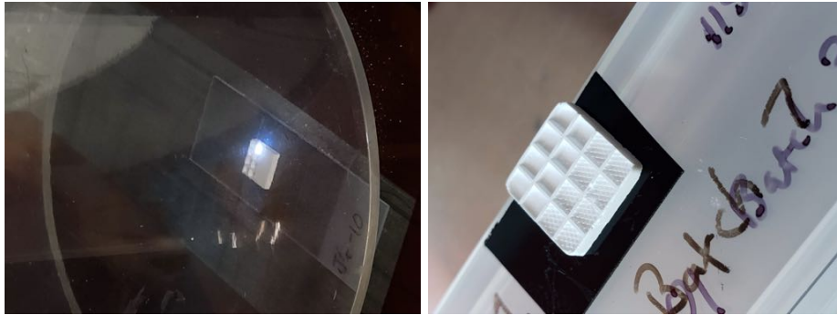
Figure 59: Left: test patterns being run on a sintered silica chip prior to thruster emitter ablation. Right: final test pattern result.
