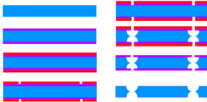
Figure 31: Insulating layer process flow. [14]
