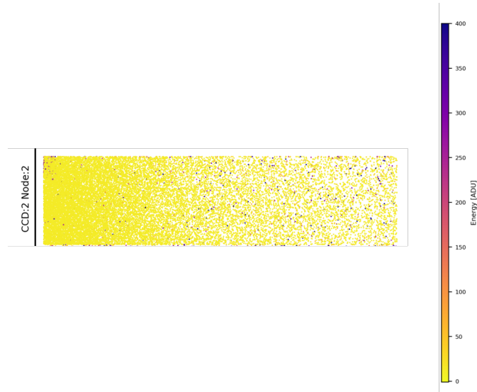
Figure 4-19: Example of event gradient across CCD22 seen throughout Orbital B
