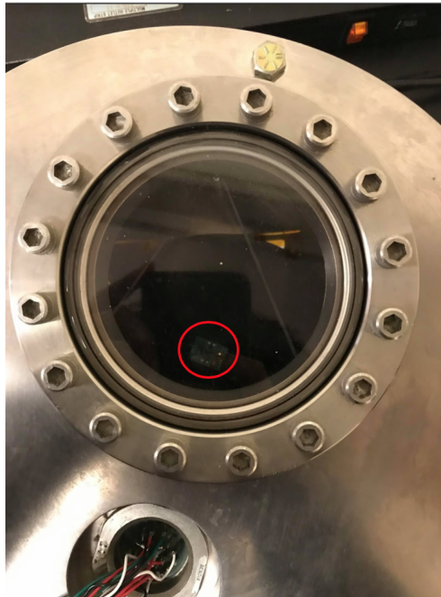
Figure 5-2: AS7262 placed unpowered in the SSL bell jar. Chamber pumped down to 19.1 mTorr
