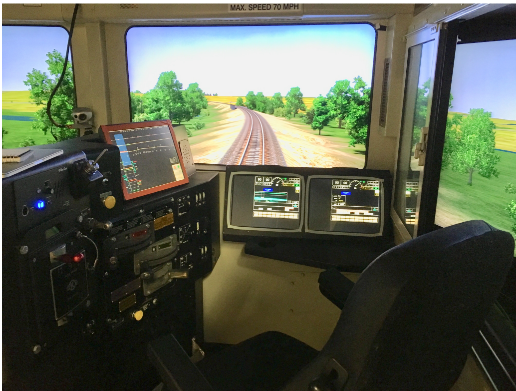
Figure 4-1: The right side of the Cab Technology Integration Laboratory, where the engineer typically sits. The control stand can be seen to the left of the seat.
