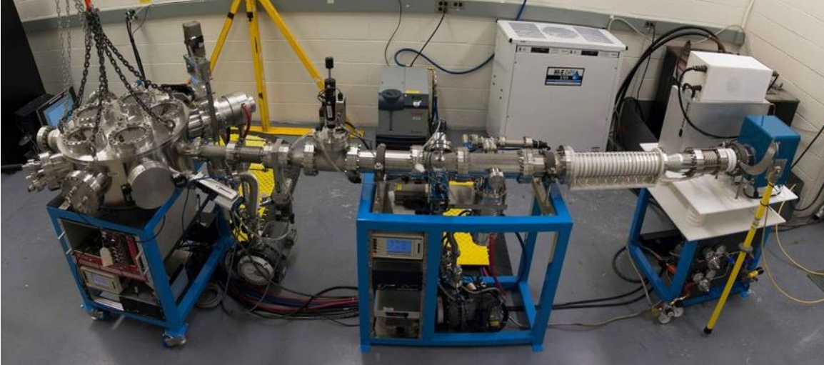
Figure 3: MIT's Linear Electrostatic Ion Accelerator (LEIA). From left to right: cylindrical target chamber, beam line, ion source (in blue shielding). Photo from Sinenian et al (2012) [10].
