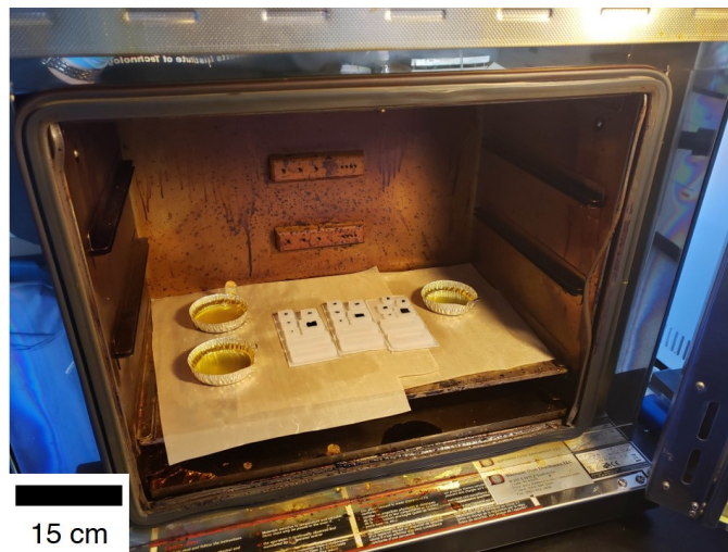
Figure 4-7: Three silicone molds with CNTs in the vacuum oven prior to infusion as part of the baseline process. Degassed resin is in the aluminum boats, ready to be poured into the molds.
