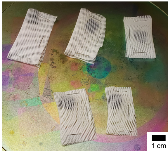
Figure 6-4: Image of A-CNT arrays prior to ALD of \text{TiO}_2 , contained in mesh for improved deposition penetration.
