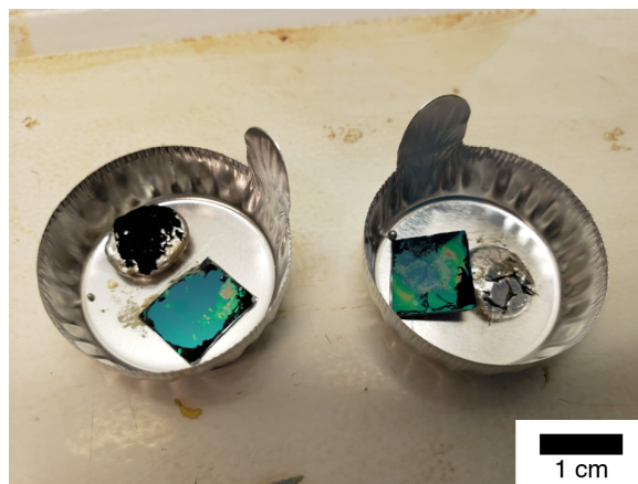
Figure 6-16: Image of successfully wetted \text{TiO}_2 -decorated A-CNTs heat treated at 700^\circ\text{C} for 30 minutes in an 80% \text{H}_2 atmosphere. Although the solder-wetted A-CNTs could be detached from the wafer, the A-CNTs were easily pulled out of the solder matrix, suggesting there was still insufficient wetting to form a true A-CNT/solder matrix nanocomposite.
