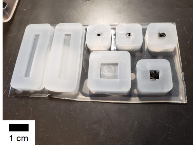
Figure 4-5: Image of A-CNT arrays ranging from 5% to 30% v_f placed in a silicone mold.
