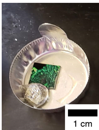
Figure 6-17: Image of unsuccessfully wetted A-CNTs with surface modification (reduced at 1000^\circ\text{C} for 90 minutes in an 80% \text{H}_2 atmosphere), demonstrating variability in the process.
