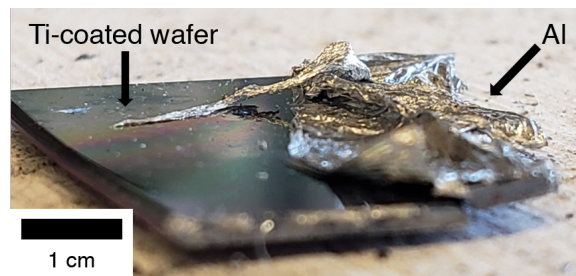
Figure 6-18: Ti-coated Si wafer wetted with molten Al. The Al spread well across the wafer, suggesting that Al will wet the Ti-coated A-CNTs.
