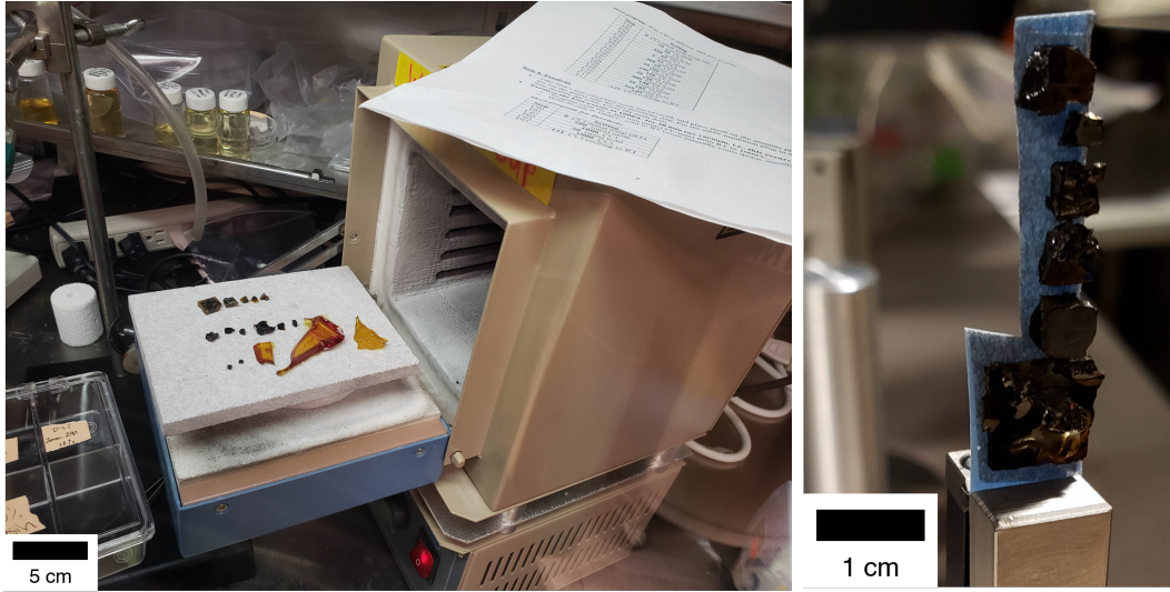
(a) A-PNCs prior to pyrolysis using improved procedures. (b) A/C-NCs after pyrolysis as prepared for \mu CT.
