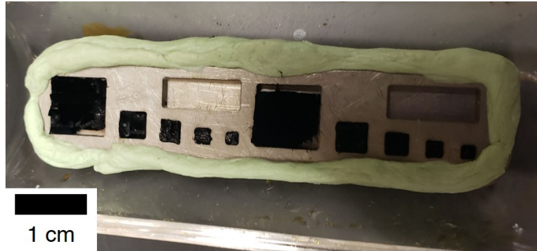
Figure 4-6: A-CNT arrays: 1% v_f (left), then 5%, 10%, 20%, and 30% v_f (right, prior to second set). A-CNT arrays were placed in the steel mold and sealed with vacuum tape prior to P-F resin infusion.
