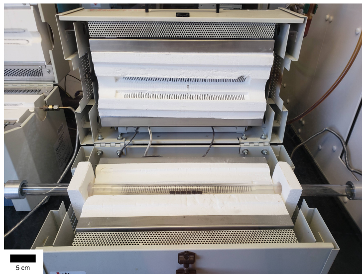
Figure 4-1: Image of six Si wafer growth substrates in the growth furnace prior to A-CNT array synthesis.
