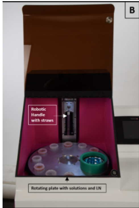
Figure 1-17: Picture of the SARAH platform. Note that the most of the small plates contain CPA solutions, and the large, green plate contains liquid nitrogen [72].
