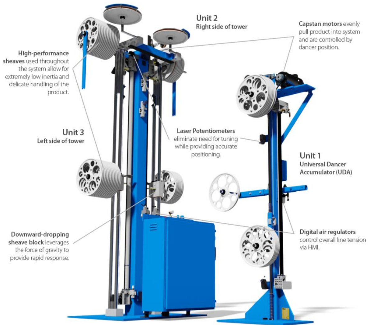
Figure 15: Example of an industrial linear tension control accumulator (Courtesy of REELEX Packaging [19])
