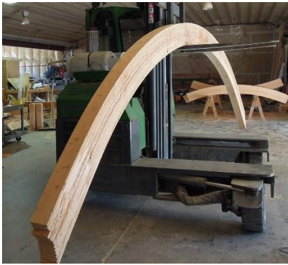
Figure 1. Forced curvature in timber through cambering (Daizen Joinery)
