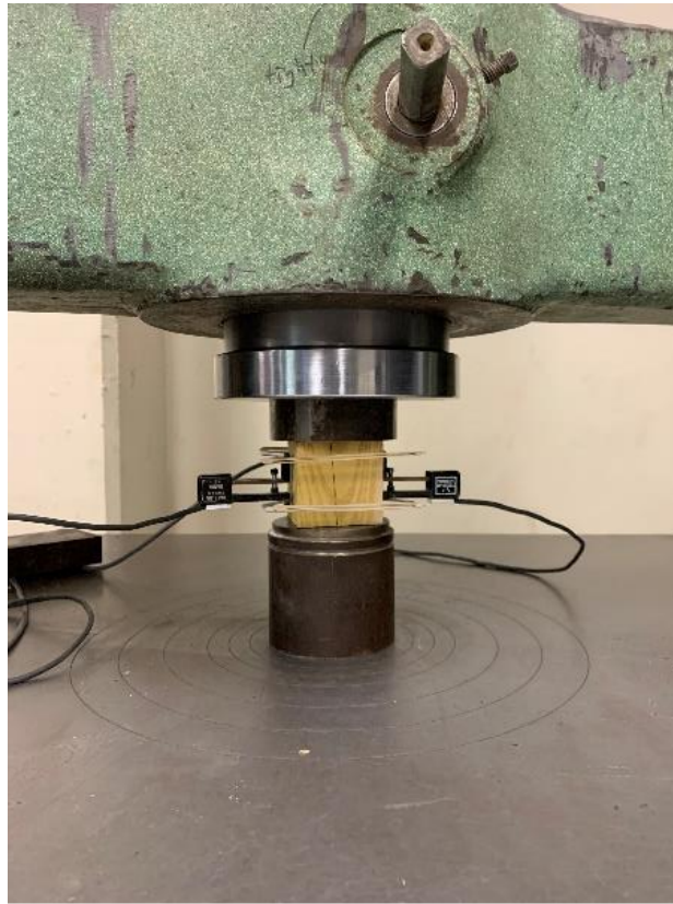
Figure 49. Cube setup -- strain gauge attached
