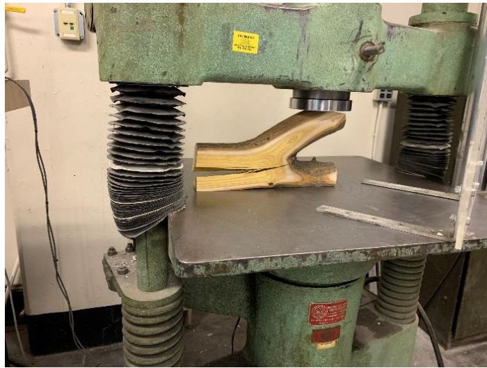
Figure 50. Cracking (top: fruit) and splitting (bottom: ash) in the non-forked branch
