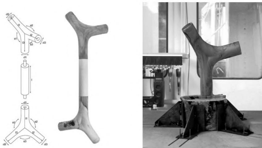
Figure 12. Standard set of tree fork elements components and assembled (left). Processed and milled tree fork (right). (Von Buelow, Peter, et al. 2018, 2)
