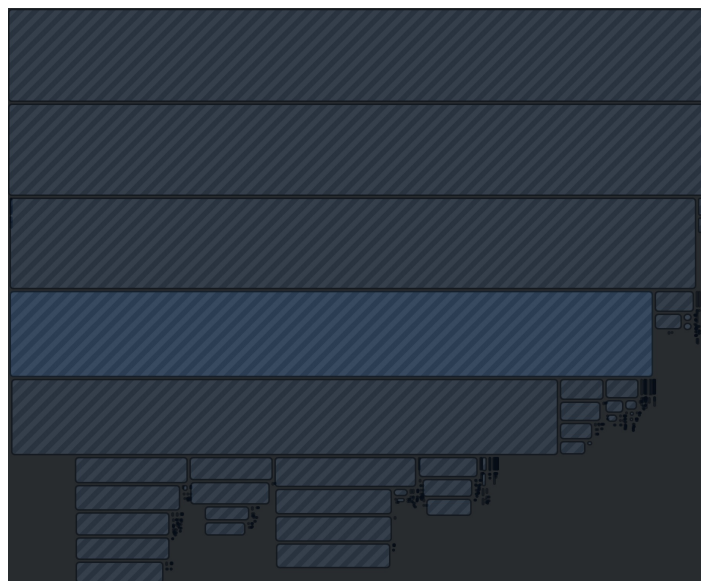
Figure 3.2: Flame graph produced through Profile.jl . The graph is a visual depiction of the number of clock-cycles per process in the program. The most time consuming computations all deal with building the model: creating variables, and adding them into the model.
