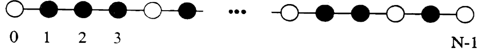
Figure 3-9: A sample path of a 1-D Ising process is shown. The process can take on two states or spins , represented above by empty and filled circles.
