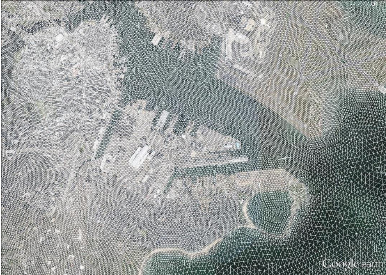
Figure 6: Boston Harbor Flood Risk Model (BH-FRM) high resolution mesh grid in Downtown Boston, South Boston, East Boston, and Inner Boston Harbor (Bosma et al., 2015).
