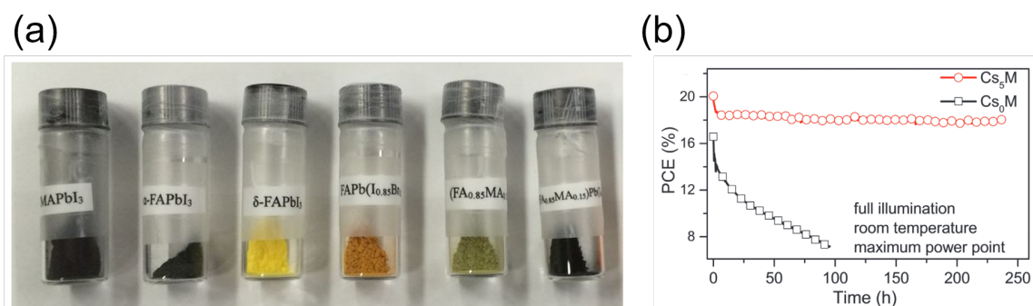
Figure 1-15: (a) Photograph of various lead halide perovskite powders. The right most sample, (\text{FAPbI}_3)_{0.85}(\text{MAPbBr}_3)_{0.15} , demonstrates the phase stabilizing effect of \text{MAPbBr}_3 for \alpha -phase \text{FAPbI}_3 perovskite. Adapted with permission from ref[8]. Copyright (2015) Springer Nature. (b) Plot of PCE versus time for perovskite solar cell with and without Cs in its composition. The device with Cs exhibits higher efficiency and improved stability. Ref[9] - Published by The Royal Society of Chemistry.
