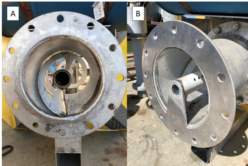
FIG 86 (A) The cantilevered end of the co-axial auger before the support bearing was added (note the damaged interior of the aluminum pipe from the impact of the unsupported steel auger). (B) The support bearing comprised a simple waterjet piece of aluminum that was caulked and bolted between the inlet device and the z-axis. The plate supported an oil-impregnated bushing that inserted into the center tube of the previously unsupported end of the co-axial auger.
