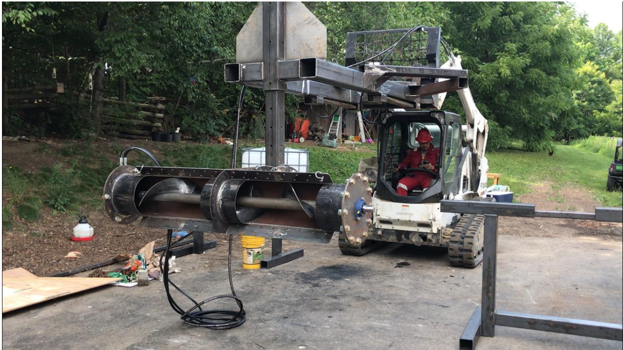
FIG 54 An early deployment mechanism for the inlet devices when the team was considering mounting the equipment on the bow of a barge. The inlets were held inside an adjustable z-axis on a frame that was forked by a skid-steer, which could also be used as an HPU for the augers.
