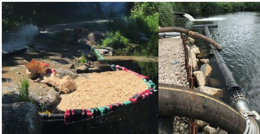
FIG 50 Different pump inlet prototypes tested from March-June 2019. (Clockwise) Co-axial auger, transverse auger, suction boom, suction tee, repurposed snowblower.
