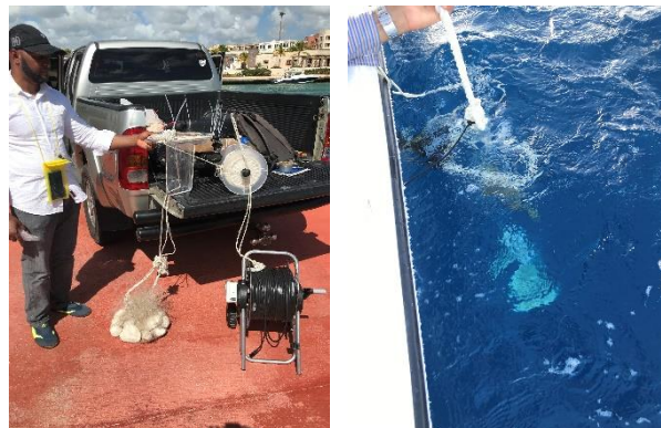
FIG 25 Left, the open-bottomed cylinder, affixed drop camera, video cable, and added weight. Sargassum was inserted into the open-bottomed cylinder and lowered below the free surface while video was captured to identify a critical depth where buoyancy is lost and the sargassum exits the cylinder.
