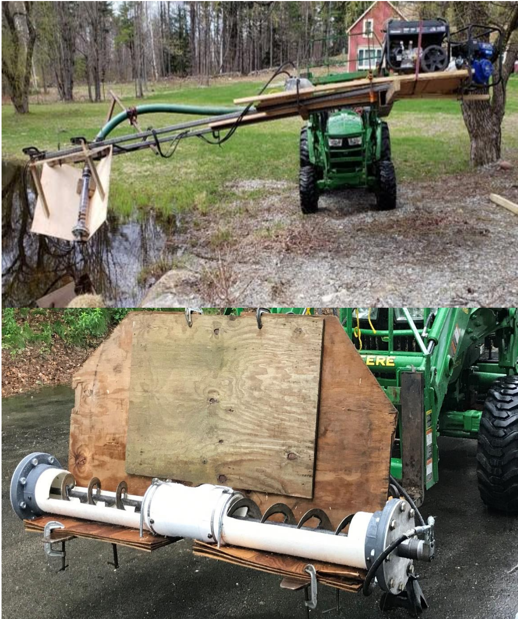
FIG 42 Prototypes of the co-axial and transverse auger devices tested using pine shavings as a surrogate for sargassum.
