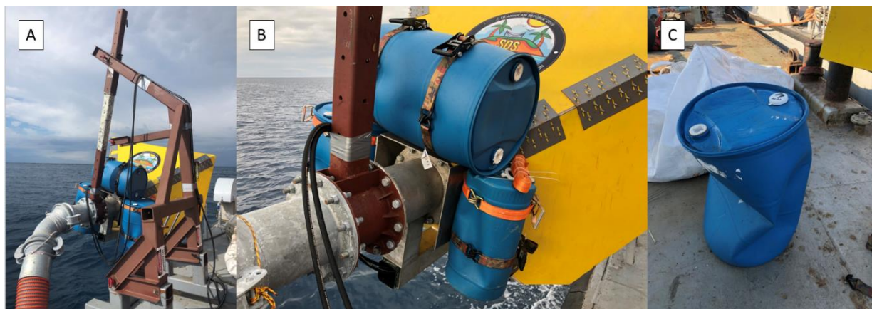
FIG 82 (A) crane and coaxial inlet in the “up” position on the portside of the GC-111 during transit (note the yellow chain grease on the z-axis for reducing resistance to linear sliding during wave-following), (B) close-up of the suction hose/z-axis/inlet device 12-bolt connection (note the 55-/30-gallon tanks strapped into vees formed by the funnel panels and aluminum plates), (C) a tank that wasn't properly sealed with silicone and was crushed in operation by hydrostatic pressure.
