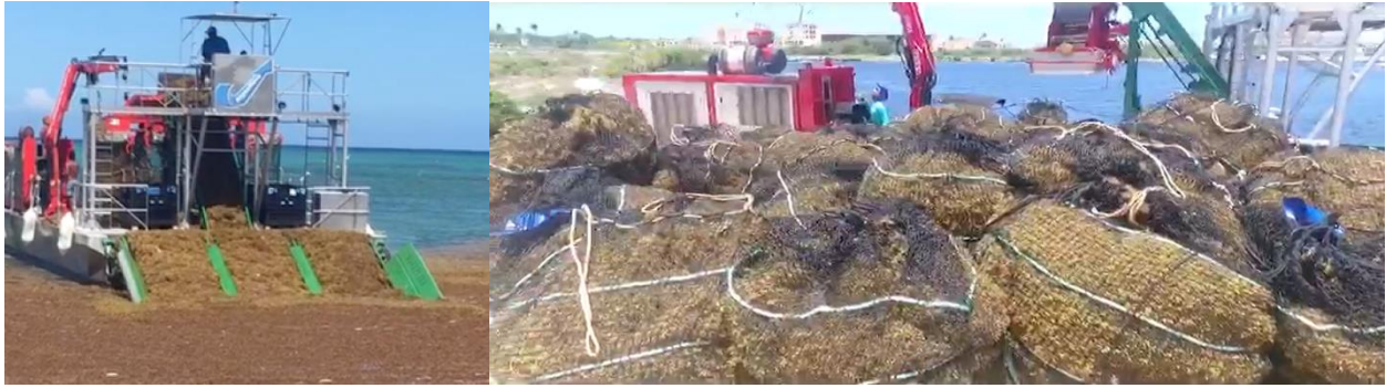
FIG 8 One of 2 specialty collection barges operated by AlgeaNova (local company) in Punta Cana, DR. This aluminum barge cost ~$400,000 to construct and requires regular overhaul of the conveyors (foreign engineers from manufacturer must service) because of corrosion from saltwater and sargassum.
