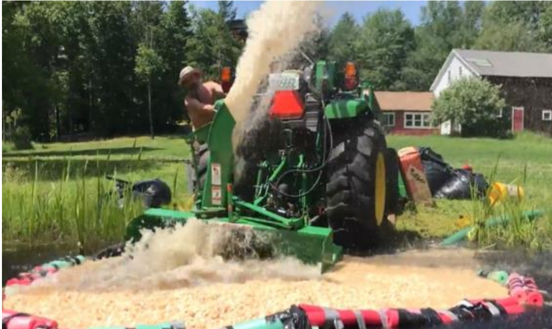
FIG 49 A test using a commercial snowblower to impel sargassum from the surface.
