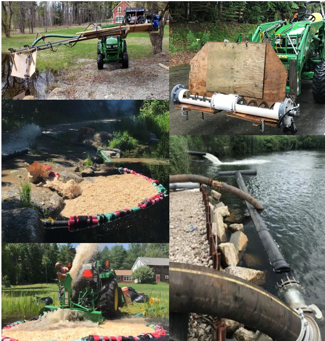
FIG 41 Different pump inlet prototypes tested from March-June 2019. (Clockwise) Co-axial auger, transverse auger, suction boom, suction tee, repurposed snowblower.
