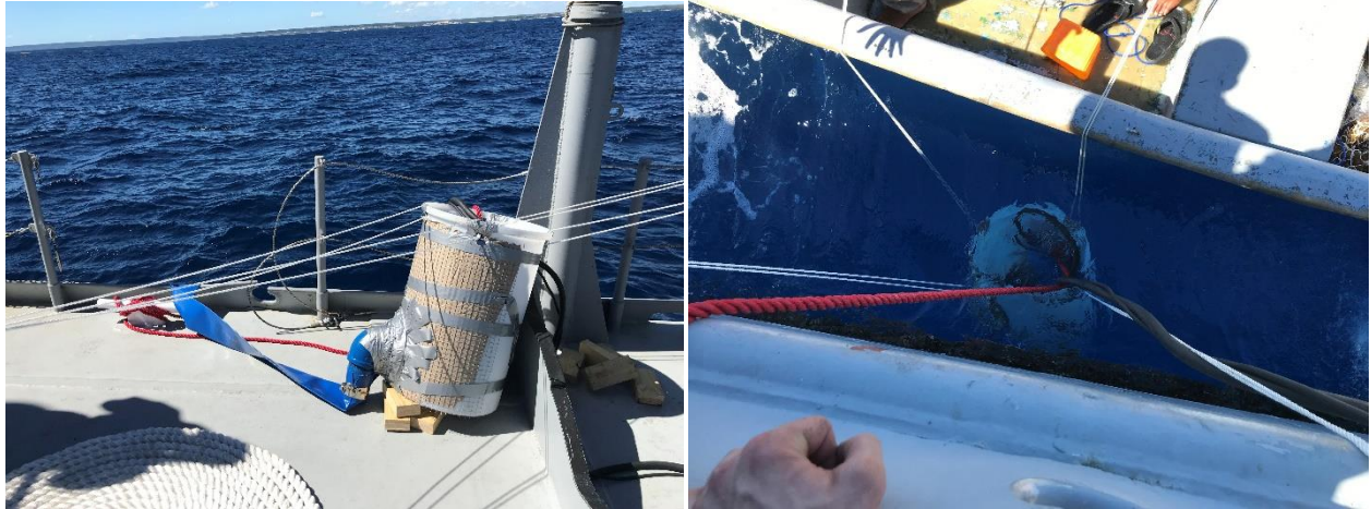
FIG 31 (Left) The sump-inlet prototype, wherein the slurry pump sits. Seawater and sargassum flows into the device from the top and exits through the hose in the base (already deployed over the starboard side of the boat). (Right) During open ocean pumping experiments, the sump-inlet prototype was suspended between a Dominican Republic Navy ship and a small artisanal boat, its depth in the water being controlled by hand, through short tethers.
