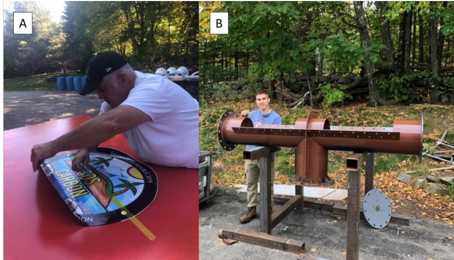
FIG 64 (A) Bob Gray applying SOS Carbon decals on the funnels of the inlet devices, (B) Luke Gray priming the transverse auger inlet device.
