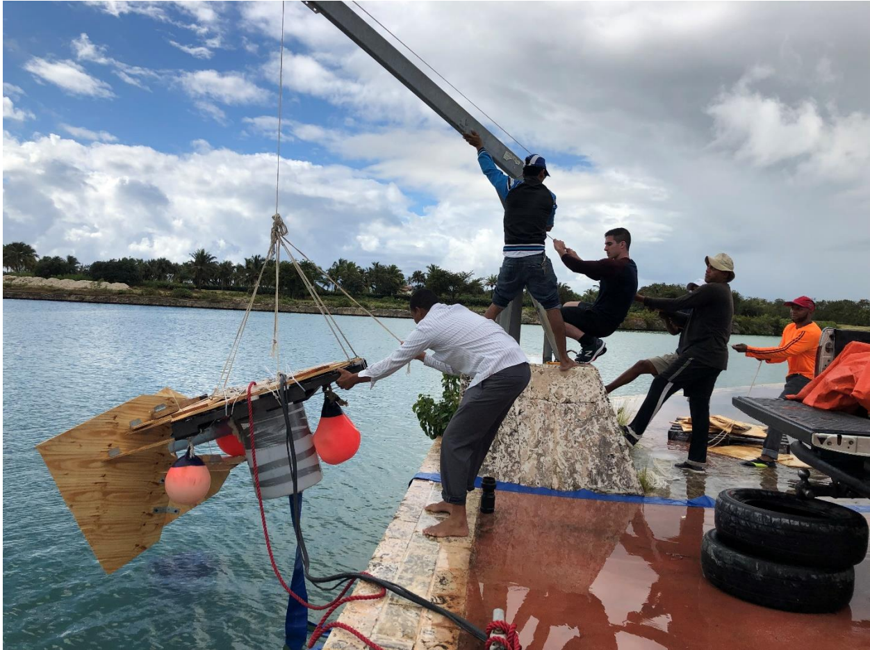
FIG 34 The combined sump-inlet/chute-inlet prototype being deployed in the back of the Marina at Cap Cana. This device allowed the observation of both the stationary sump-inlet and the moving chute-inlet dynamics with the same wet-pit pump installation inside the sump.
