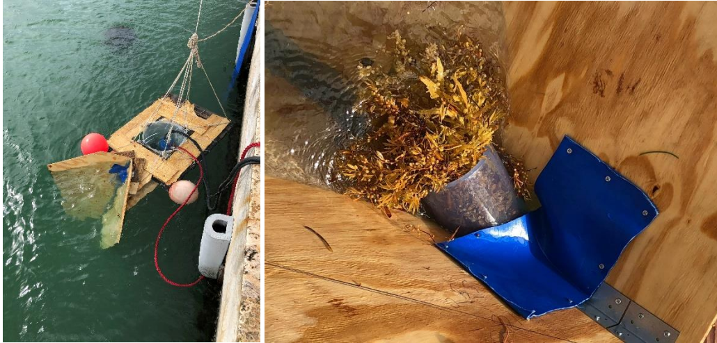
FIG 36 (Left) Video captured of the moving “chute-inlet” in the calm waters at the back of the Cap Cana Marina. The chute-inlet was pulled along the marina wall as sargassum was thrown into its path. (Right) A clog that developed at the inlet piping due to the low suction exerted. This risk will be remedied with an auger in the future.
