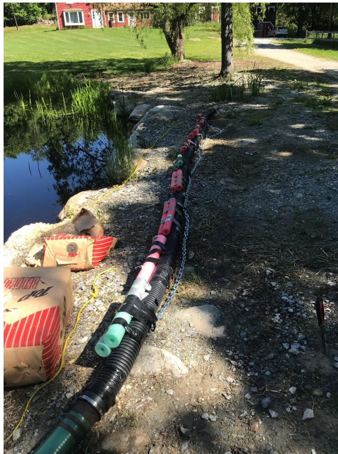
FIG 51 Prototype version of the suction boom (flexible), showing the chain ballast used to counteract forces from waves and flow of water through the boom.
