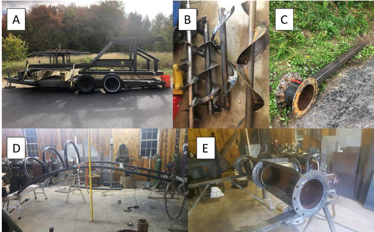
FIG 61 (A) finished weldments of the hose reel (base and wagon-wheel) arriving at Prof. Slocum’s farm, (B) 2ea 48” coaxial augers (spoked and solid) and 2ea 80” transverse augers (spoked and solid), (C) the z-axis that rides inside the rotating sleeve on the end of the crane and connects the inlet devices to the suction hose, (D) the stinger for guiding the hose over the dive deck on the back of the GC-111 Centaurus, (E) the transverse inlet device.
