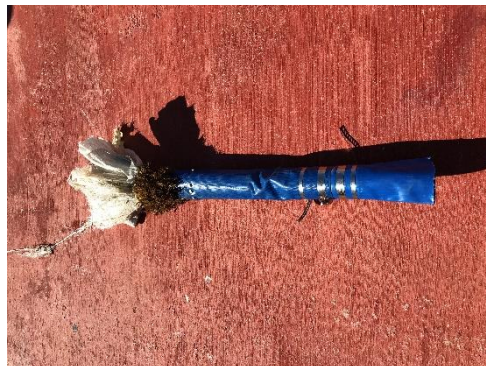
FIG 33 The severed end of the hose used during the open ocean pumping experiments. A clog developed at the terminus of the hose, at the end of the pumping experiment, due to the concentrated fixturing, as well as the proximity of the affixed weight, at the end of the hose. There were no other clogs along the entire length of the hose.
