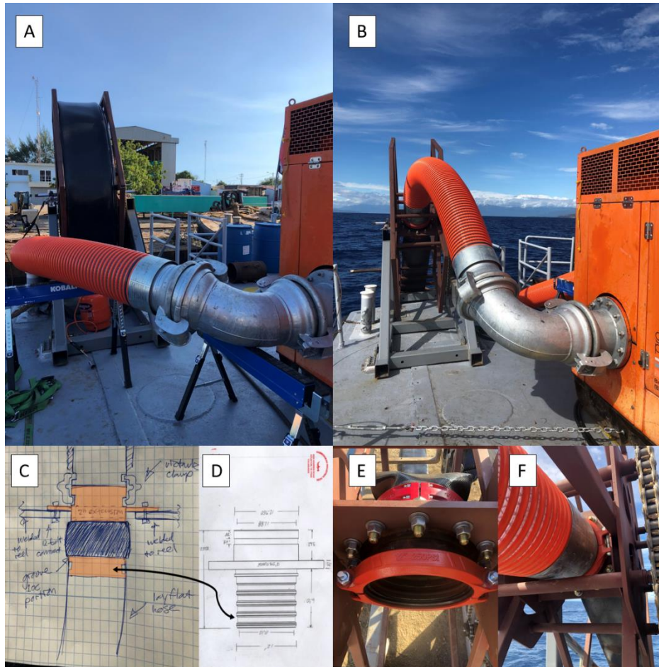
FIG 87 (A) the pilot at mooring with the layflat hose completely reeled up and the discharge kanaflex hose from the pump left disconnected, (B) the pilot vessel at sea with the layflat hose completely unreeled and the discharge kanaflex hose connected to the layflat hose via a custom fitting in the center of the hose reel, (C) L. Gray's original drawing indicating the changes needing to be made to the layflat hose vendor's off-the-shelf hose fitting, (D) the layflat hose vendor's dimensioned drawing for the custom fitting, showing how an off-the-shelf hose fitting would be cut and a \frac{3}{4} " 12-bolt IPS flange would be welded in the middle, (E) a close-up of the custom layflat hose fitting, bolted to a plate in the center of the hose reel, with a Victaulic groove/clamp extending from the opposite side such that the kanaflex discharge hose (from the pump) could be connected, (F) a close-up of the connection between the kanaflex discharge hose and the 200m layflat hose, via the custom layflat hose fitting bolted to the center of the hose reel.
