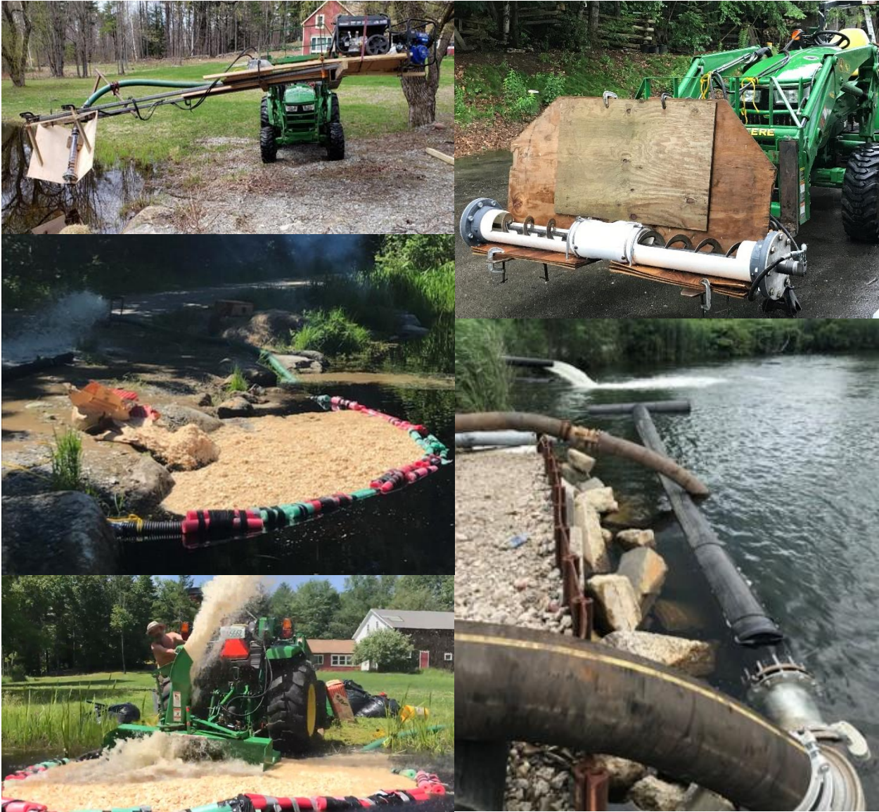
FIG 3 Different pump inlet prototypes tested from March-June 2019. (Clockwise) Co-axial auger, transverse auger, suction tee, repurposed snowblower, suction boom. The moving auger devices (coaxial and transverse) were chosen for full-scale design.
