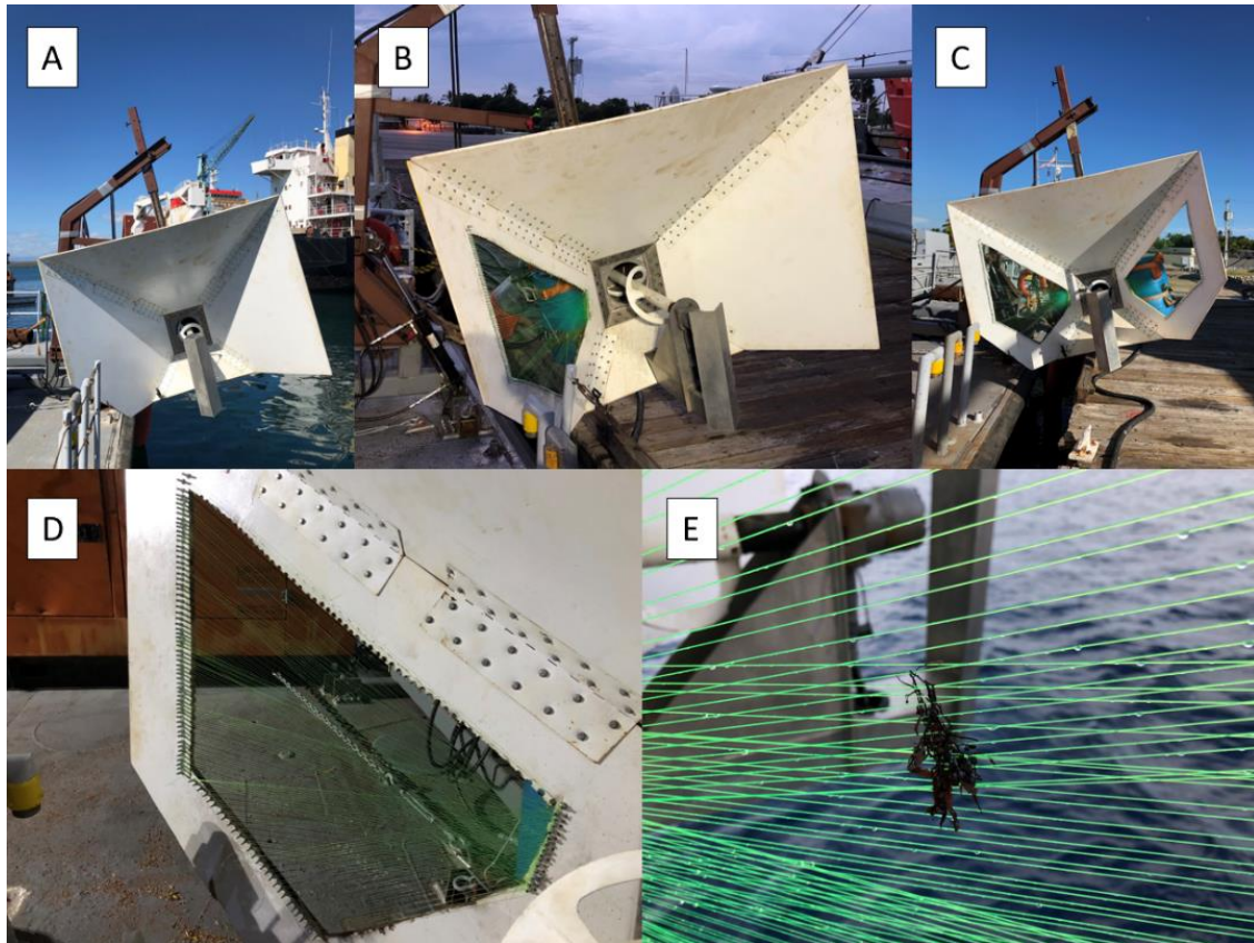
FIG 95 (A) solid funnel prior to pervious modification being made, (B) the funnel with one side made pervious, (C) the funnel with both sides made pervious, (D) a close-up of the radially symmetric weave of high-strength fishing line, (E) a close-up showing the tightness of the weave of fishing line, compared to a small fragment of sargassum left after testing one day.
