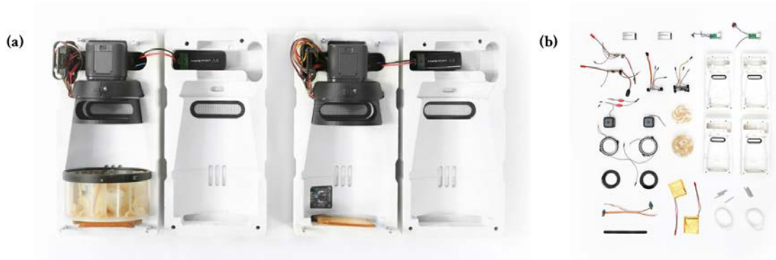
Figure 14: (a) Two-part foam design, two identical autonomous Nanolabs (A and B) were produced for the flight. Controls were performed in separate settings using foam parts of the same type and color. (b) All parts of the Nanolabs.
