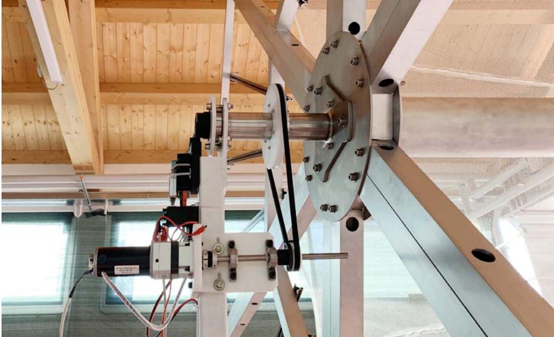
Figure 35: Motor and belt drive system.
