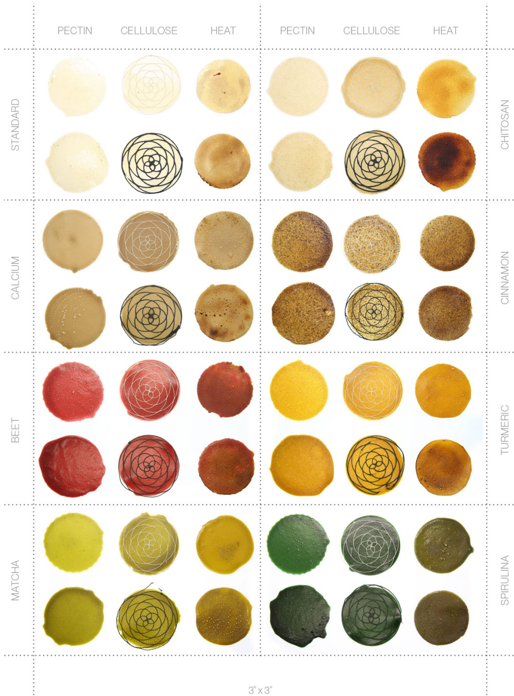
Figure 24: Matrix of O swatches showing tunable variation in material qualities using different pectin formulas, toolpaths, printing methods, heat and air exposures.
