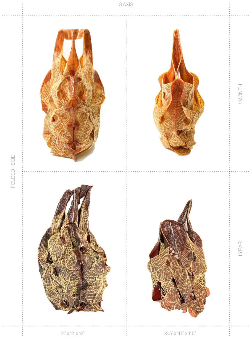
Figure 83: Matrix of Y Fold – Multiple geometries exposed to air over 1 year comparing color change and deformation of 3-dimensional form.
