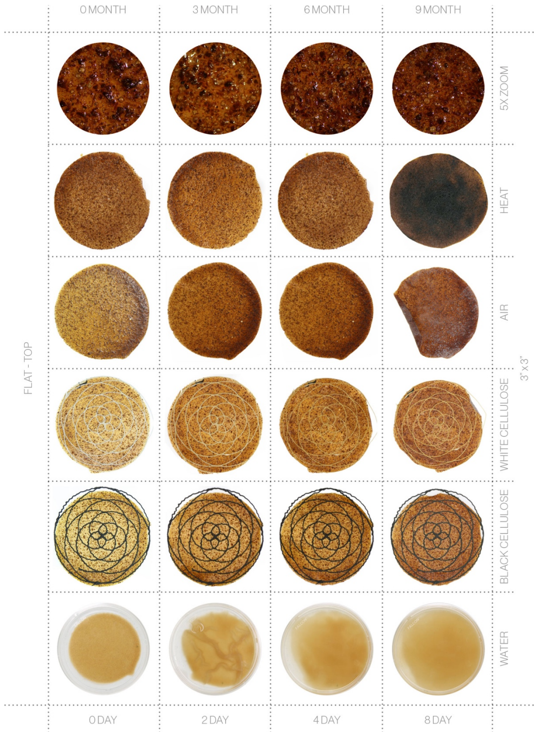
Figure 51: Matrix of O Swatch - Cinnamon pectin formula comparing color change and deformation in response to exposure to heat, air and moisture over time.
