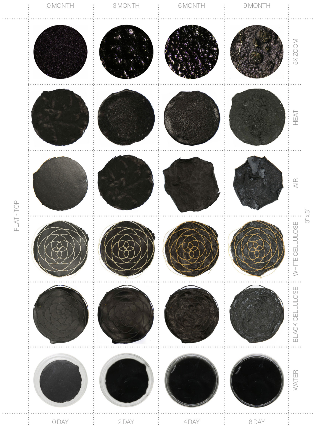
Figure 57: Matrix of O Swatch - Charcoal pectin formula comparing color change and deformation in response to exposure to heat, air and moisture over time.
