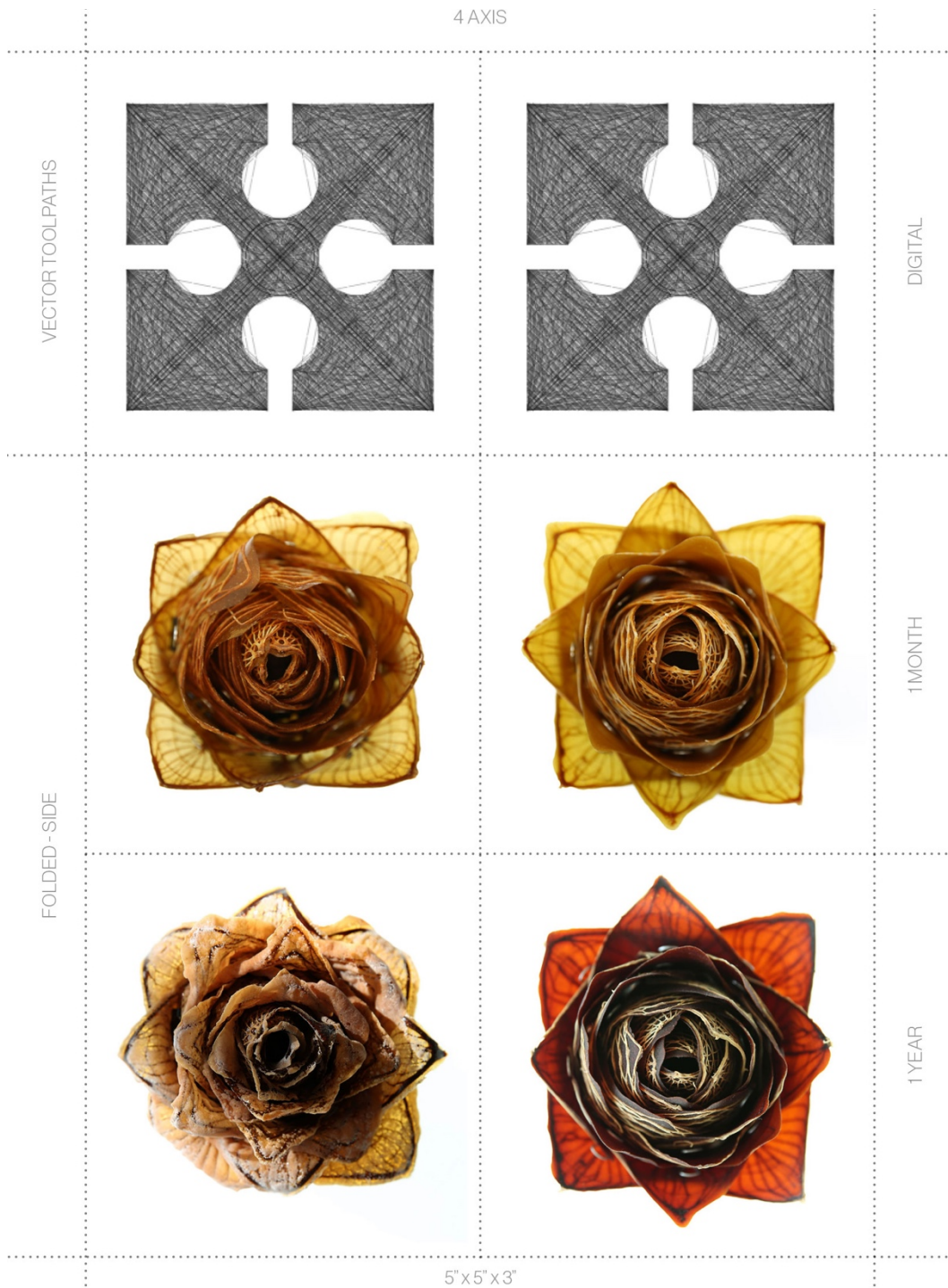
Figure 27: Comparison of the deformation of X flower prints aged over 1 year with (left) pectin/chitosan and cellulose composition vs. (right) pectin/chitosan, cellulose, and pectin composition.
