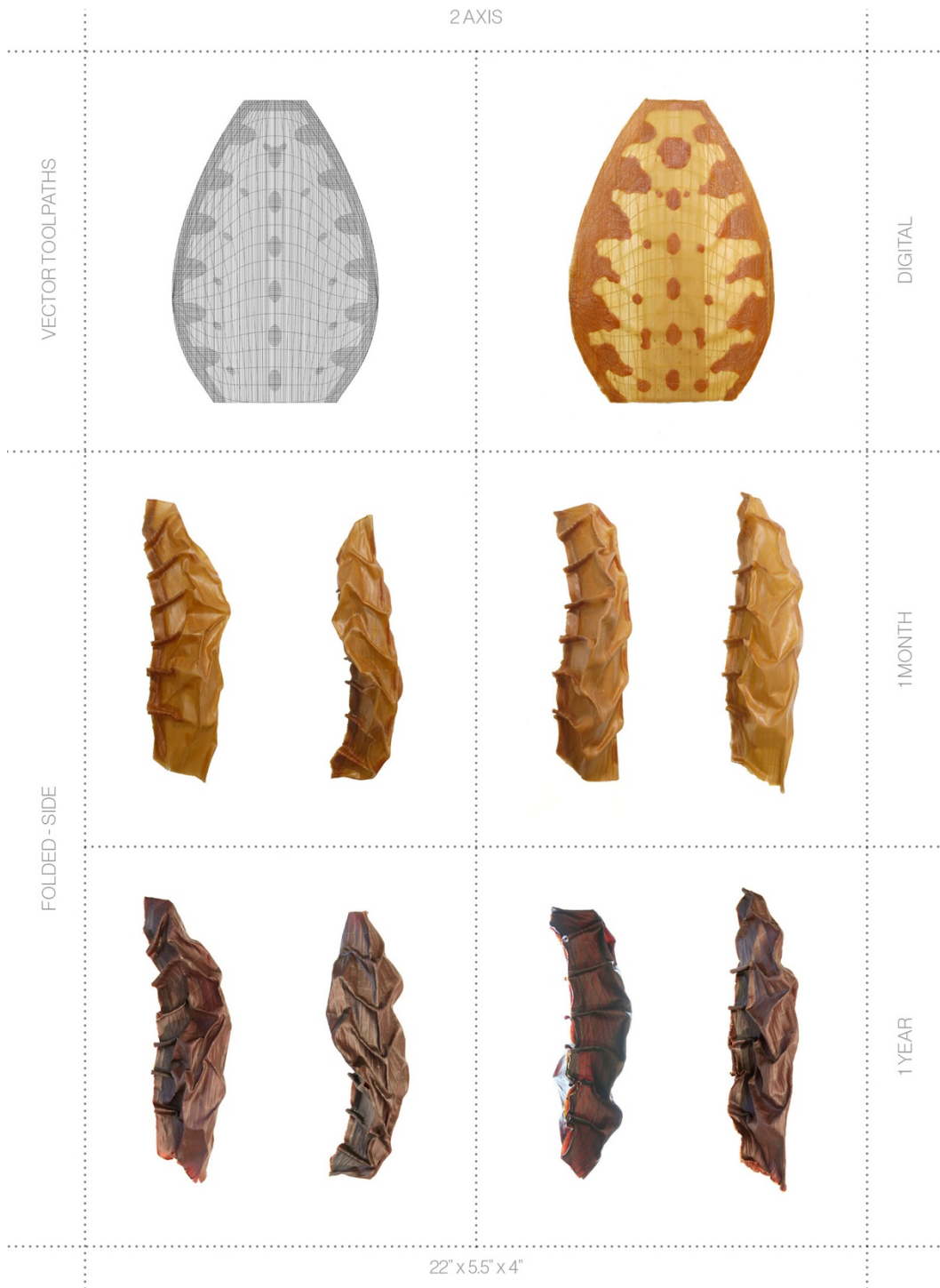
Figure 32: Comparison of the deformation and color change of I crease prints aged over 1 year with different 3-dimensional forms.
