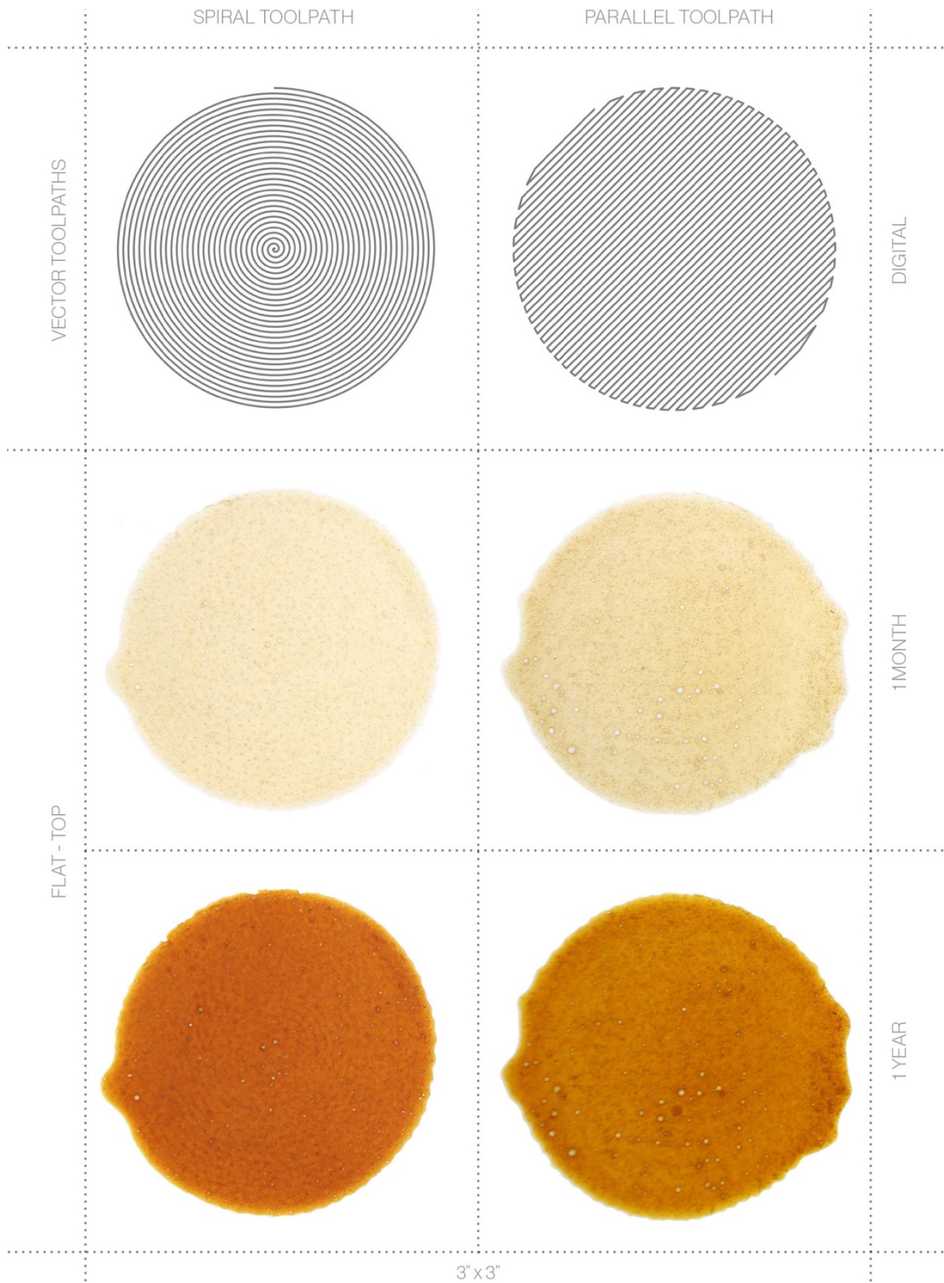
Figure 23: Pectin/chitosan mixture formula printed in circular diameter swatches with spiral and parallel toolpaths. (top) vector toolpaths, (middle) print after 1 month, (bottom) print after 9 months. 3" x 3"
