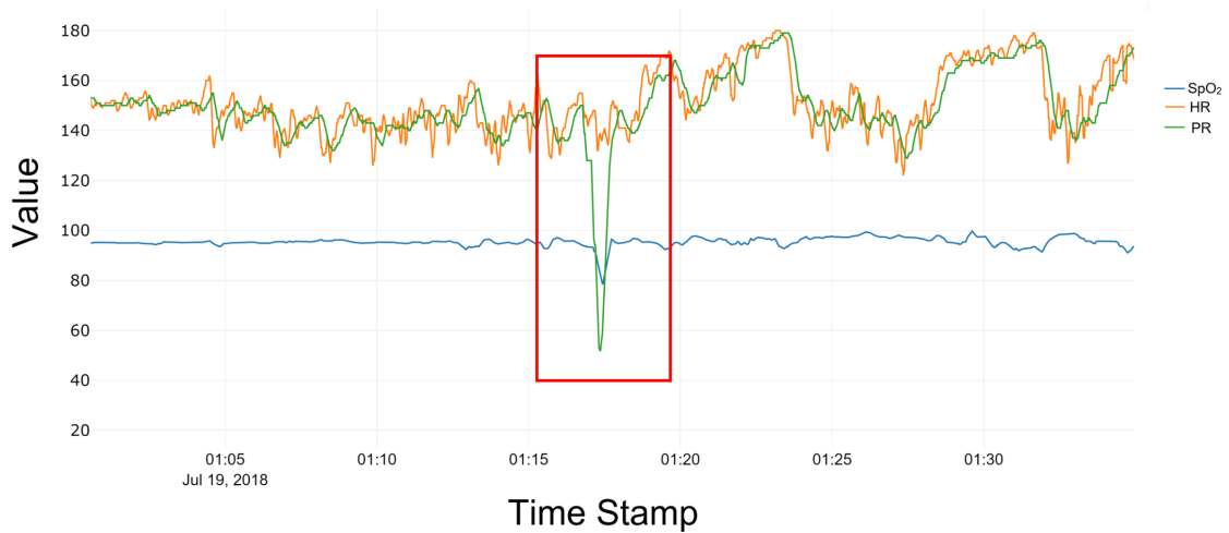
Figure 5-6: Sample SpO 2 , HR, and PR values over 20 minutes. The red box illustrates an example when HR and PR deviate by more than 10 BPM.
