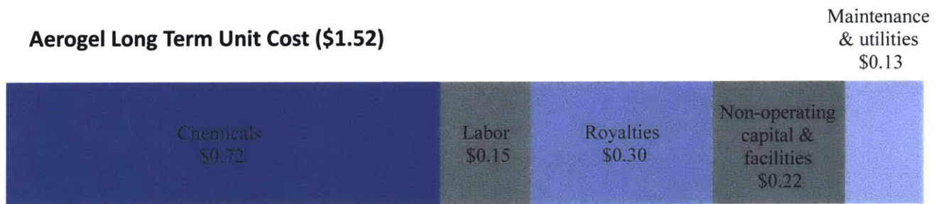
Figure 57. Unit cost of aerogel production driven by chemicals needed for production. This cost can be reached at a 4.5 million sqft production volume.
