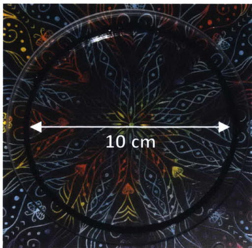
Figure 42. Double-pane window prototype using DRL aerogel. The aerogel will replace the gap traditionally filled with gas and the edge-spacers support the double-pane structure.
