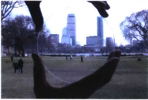
Figure 41. a) Ultra-clear aerogel sheet (6" diameter) with a porosity of 94%. Average pore and particle feature sizes are <10 nm diameter, allowing transmittance >98%, haze <2.0%, and thermal conductivity <13 mW/mK through 3 mm thickness. b) Proposed aerogel double-pane window with inset showing the ultra-clear aerogel compared to float glass. The aerogel replaces the air gap in a double-pane window.
