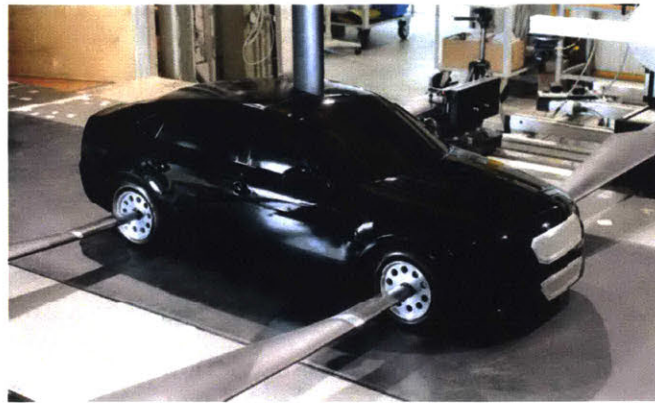
Figure 4-47: Experimental setup in the wind tunnel (from [15])
