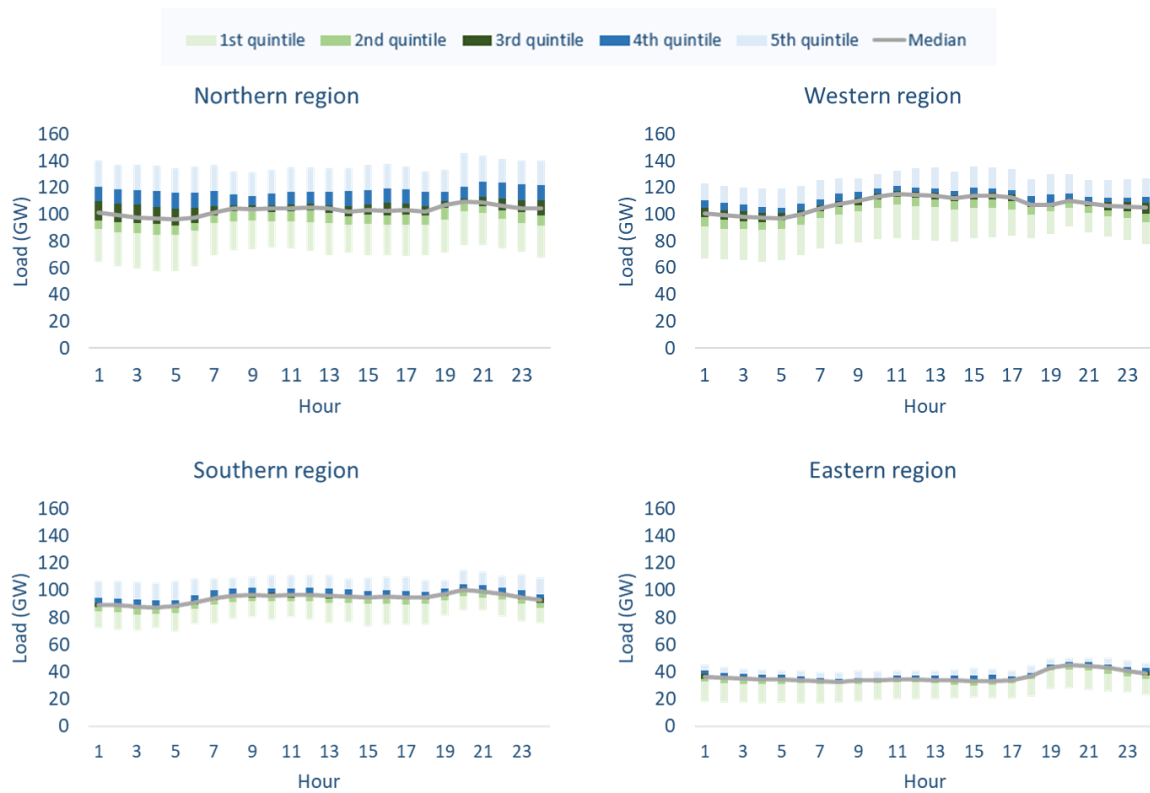
Figure B-1: Distribution of regional electricity demand per hour of the day for the year 2036-37.
