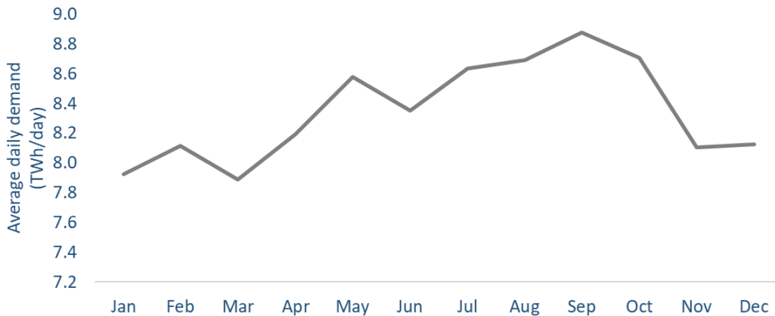
Figure 5-5: Estimated average daily load for the system per month in the year 2036-37. Source: Own elaboration based on scaling up 2015 load estimates.
