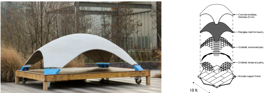
Figure 1.2: Concrete shell on elastic gridshell. In this system, the shape of the elastic gridshell must match the geometric constraints of elastic gridshells and be as close as possible to a funicular shape for the concrete shell.
