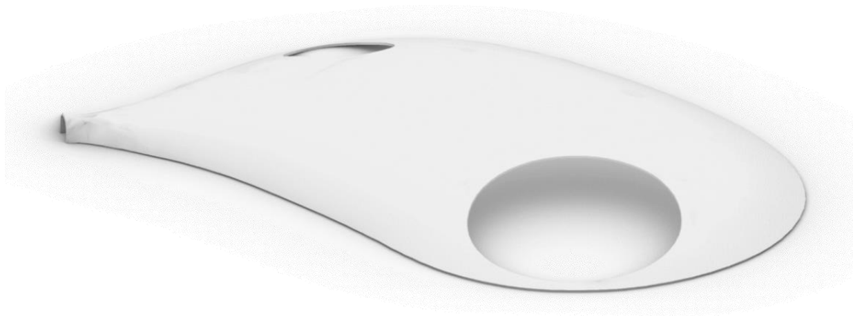
Figure 6.11: Rendering of the funicular shape obtained with this work to reproduce the Teshima museum shape.
