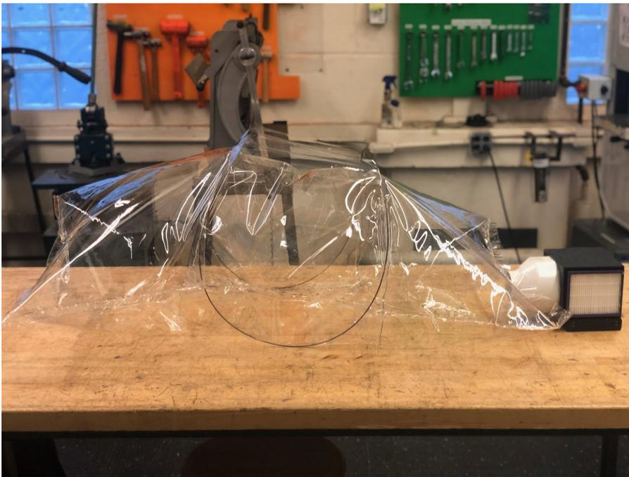
*Fig 5-14: Spring steel frame in TPU enclosure, side view. Pockets are hard to discern because they are made of the same transparent material as the enclosure.*
