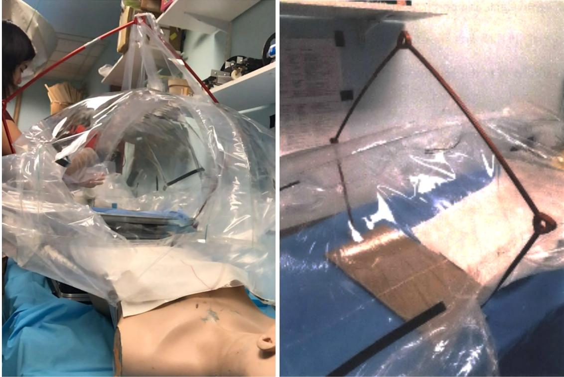
*Fig 3-5: Pentagonal support frame. The enclosure is tethered to the top of the frame using some plastic ties attached to the surface of the enclosure. As seen in the photos, the red-anodized aluminum frame members are slightly bowed under the pre-load required for assembly.*
