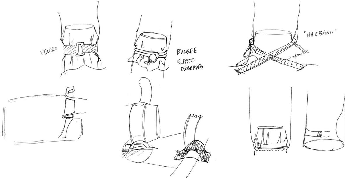
Fig 5-5: Ideation sketches of potential enclosure-box connection mechanisms
