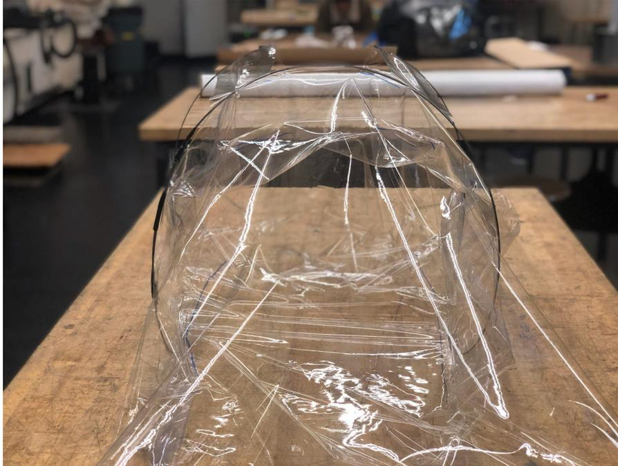
*Fig 5-13: Spring steel frame in TPU enclosure, axial view.*
