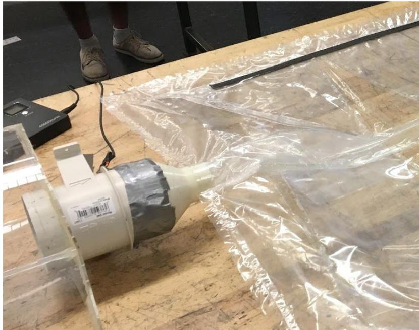
*Fig 3-4: "Slip fit" enclosure-box connection. Note the duct tape on the blower. The duct tape was used to secure the enclosure box connection on some prototypes that had loose connections.*
