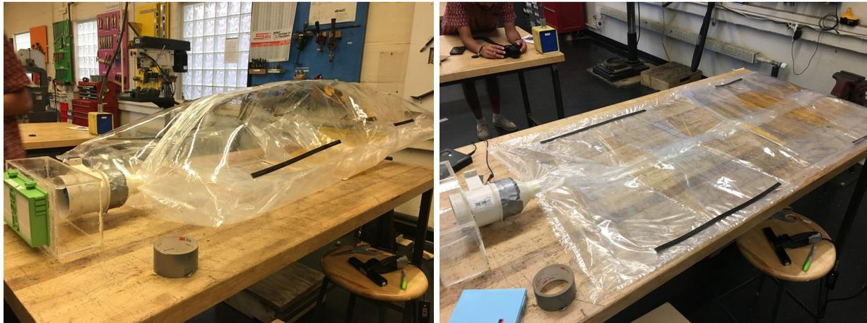
*Fig 3-1: Generation 6 SurgiBox prototype shown in inflated state (left) and deflated state (right).*
