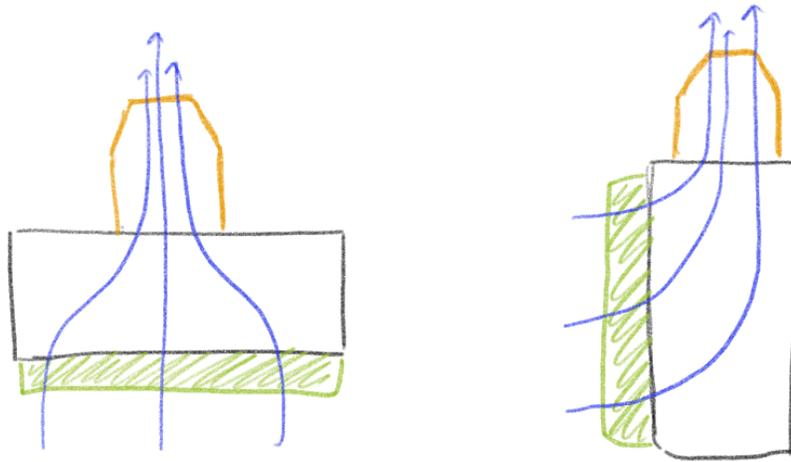
Fig 3-3: Two air filter box architectures: T-shaped (left) and L shaped (right). The filter is shown in green, nozzle shown in orange, and the airflow direction shown in blue.
