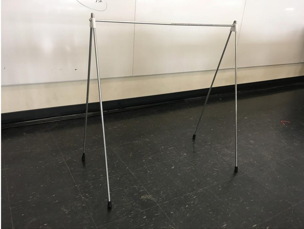
*Fig 5-7: Assembled A-frame support frame*
