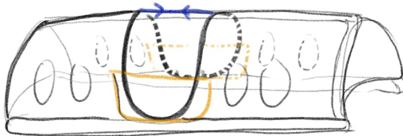
*Fig 5-12: Position of pockets for spring steel frame. Pockets are shown in orange. Single tether at the top is shown in blue.*
