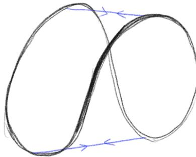
*Fig 5-10: Position of tethers for saddle shaped spring steel frame. The tethers will always be located opposite of each other, in orthogonal directions.*
