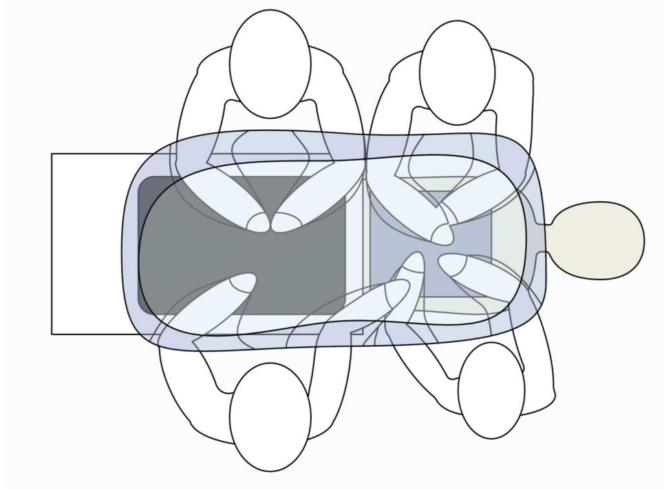
*Fig 1-1: Schematic of SurgiBox concept: a transparent enclosure positioned on the patient's torso, with sleeves for surgeons to access the surgical site.<sup>8</sup>*
