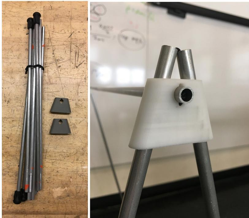
*Fig 5-8: A-frame support frame in packed configuration*
