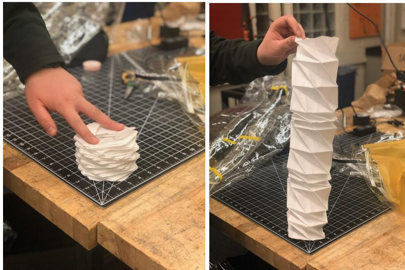
*Fig 5-4: Small scale prototype of foldable filter*
