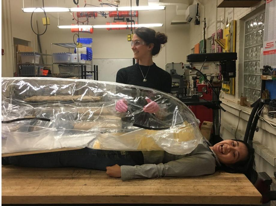
*Fig 1-3: Generation 6 SurgiBox Prototype. Note the black line on the left is where the port is. The port is sealed by two thin strips of flexible magnetic sheet, which gives it a black color.*
