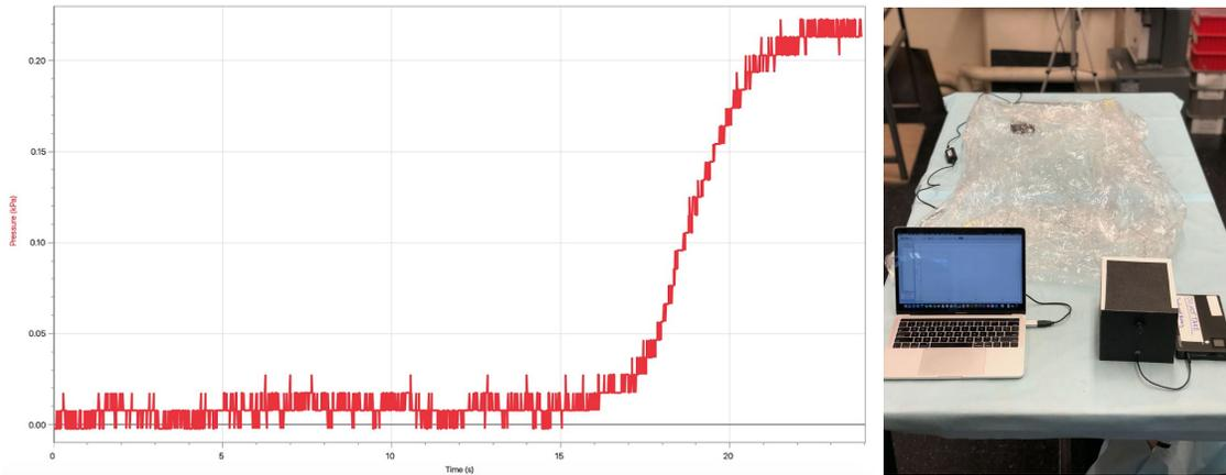
*Fig 5-2: Sample data of the filter surface area experiment, the graph shows pressure as a function of time.. The time to inflation is measured from when the slope first begins to increase, to when the slope decreases back to zero.*
