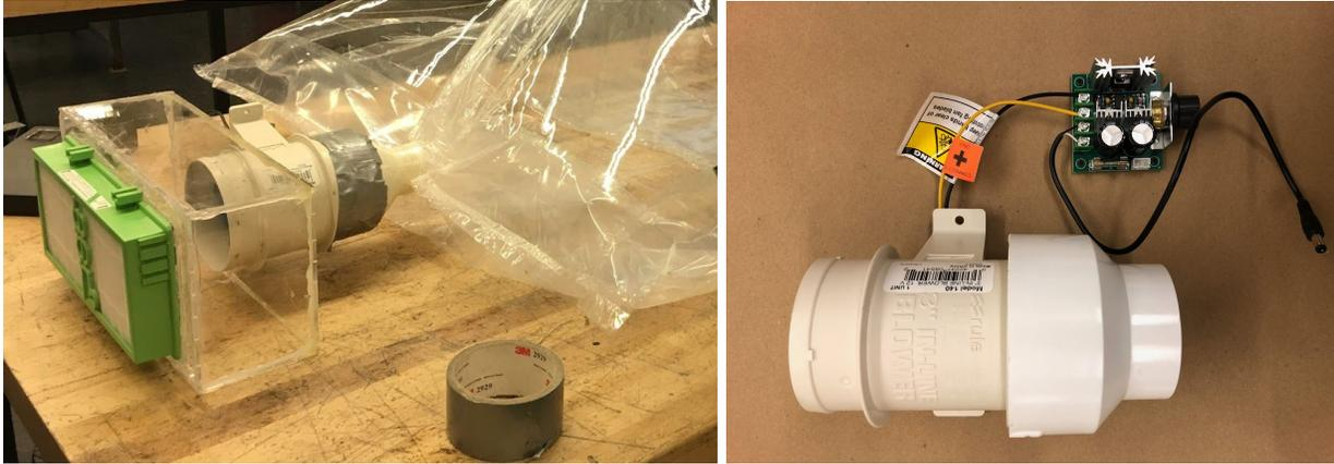
Fig 3-2: Air filter box and internal components. Full assembly (left) and blower and microcontroller carrier board (right).
