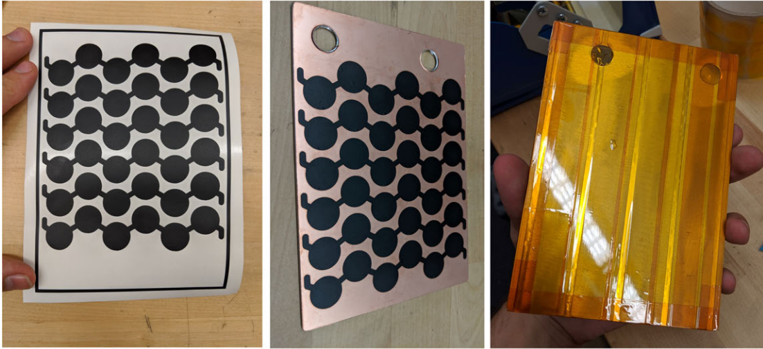
Figure 4-3: Vinyl mask cut, applied, and masking the remaining exposed aluminum.
