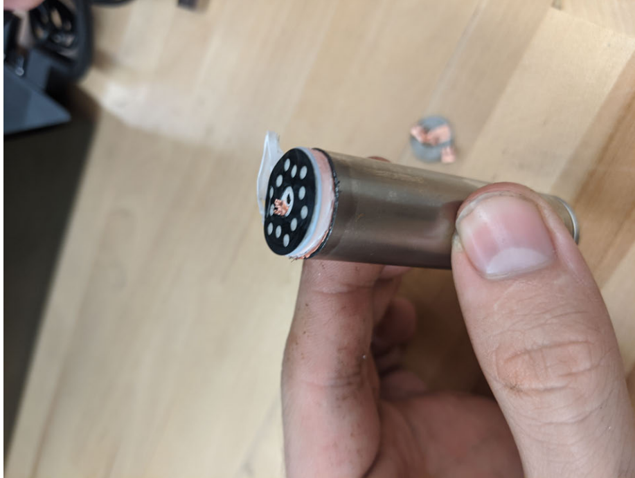
Figure 2-7: Teardown of the bottom side of the 18650 showing the anode end insulator.
