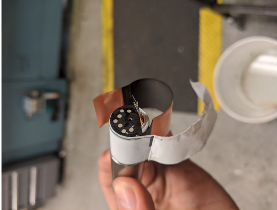
Figure 2-6: Teardown of the 18650 cell reveals the jellyroll construction and insulators on each end.
