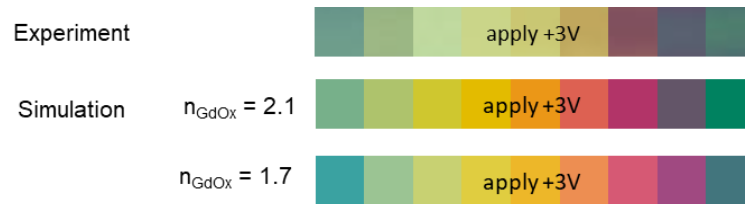
Figure 5.6. Experiment micrographs and simulated colors of yttrium gating reflection devices with different \text{GdO}_x refractive index when loaded with hydrogen. The refractive index change of \text{GdO}_x only contributes minor change to the colors.
