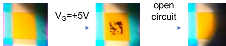
Figure 7.2. Gate voltage controlled hydrogen loading/unloading device fabricated on a chip with a 200 nm thick 0.5 mm x 0.5 mm square Si 3 N 4 window showing reversible deformation with gate voltage application.
