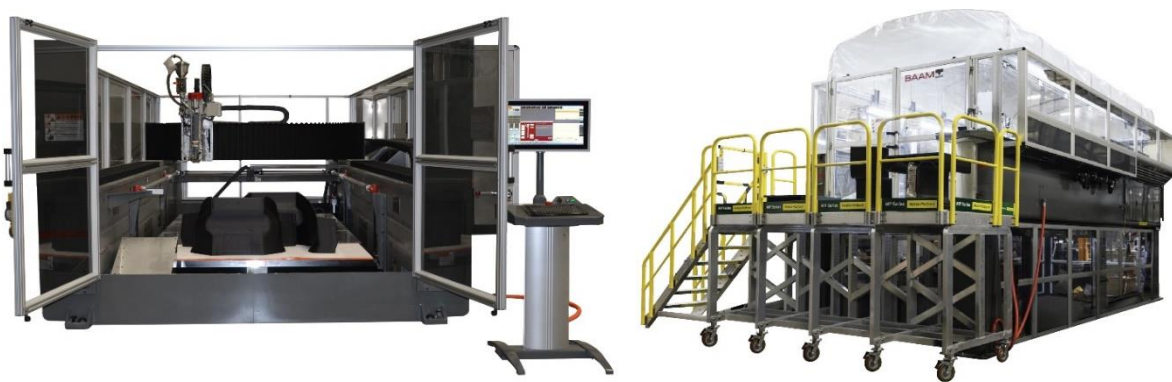
Figure 1-7: BAAM 3D printer interior (left) and exterior (right). Printing can be accomplished in a contained space and tubing conveys pellets directly into the extruder attached to the print head [23].
