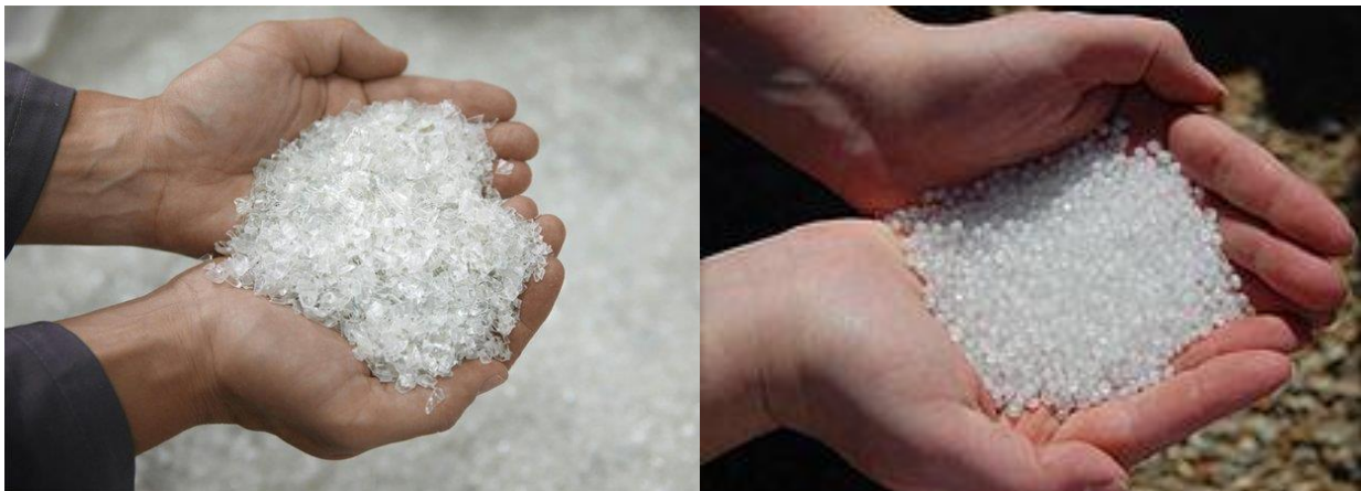
Figure 4-1: Flake size and shape (left) vs. pellet size and shape (right). Pellets are manufactured resulting in uniformity while flakes have greater variation [99,100].
