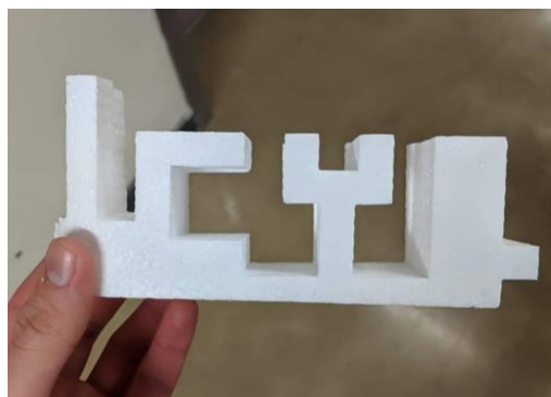
Figure 5-9: “IcyQ” letters cut out of EPP foam using the 4-axis CNC foam cutter.
