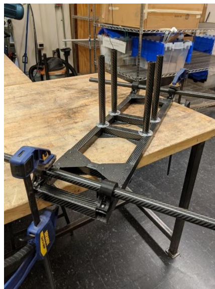
Figure 4-1: Mechanical structure of the aircraft assembled with epoxy curing.
