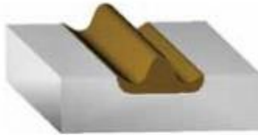
Figure 6: Image depicting a seal bonded to a metal substrate [20].
