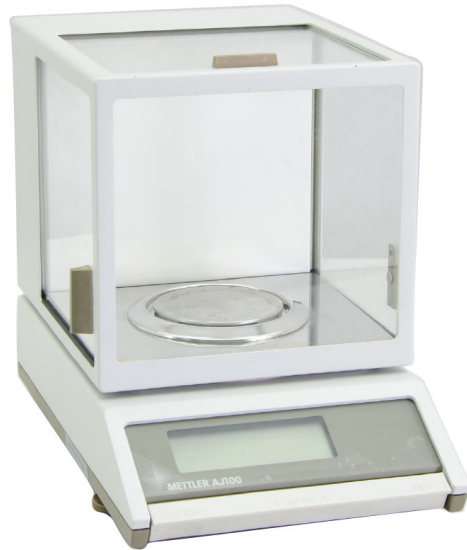
Figure 2-6: The AJ100 analytical balance used for lattice mass testing. Samples were centered on the plate, and mass was recorded with 0.001 g resolution.
