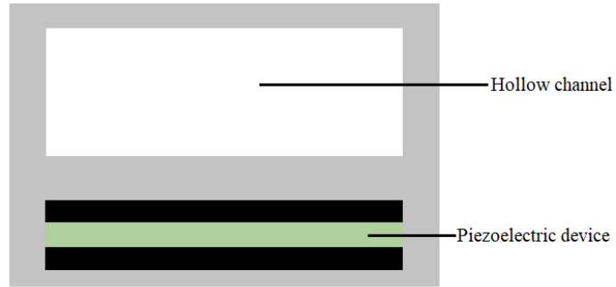
Figure 12: Cross sectional view of a potential shape change for the future study. The hollow channel at the top is an attempt to act as a sound-amplifying channel, resembling that in a bell stethoscope.
