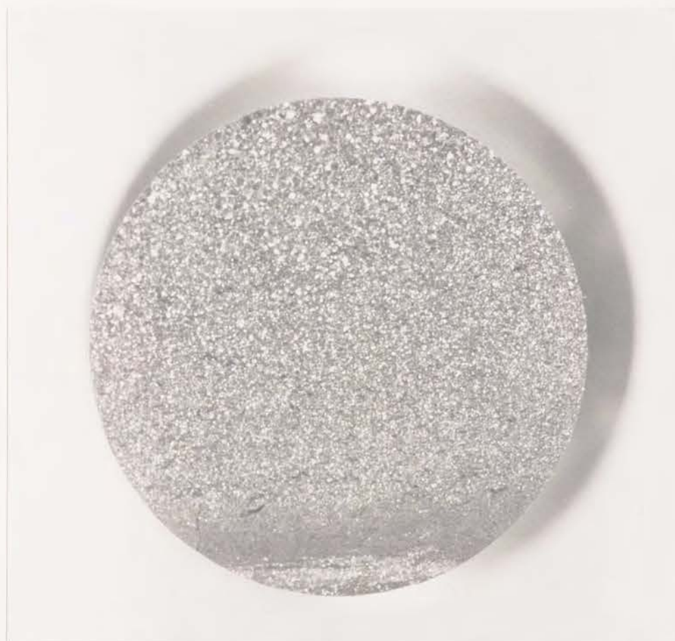
Figure 13: Fracture surface of a tensile test bar. Note variation in structure. 5X.
