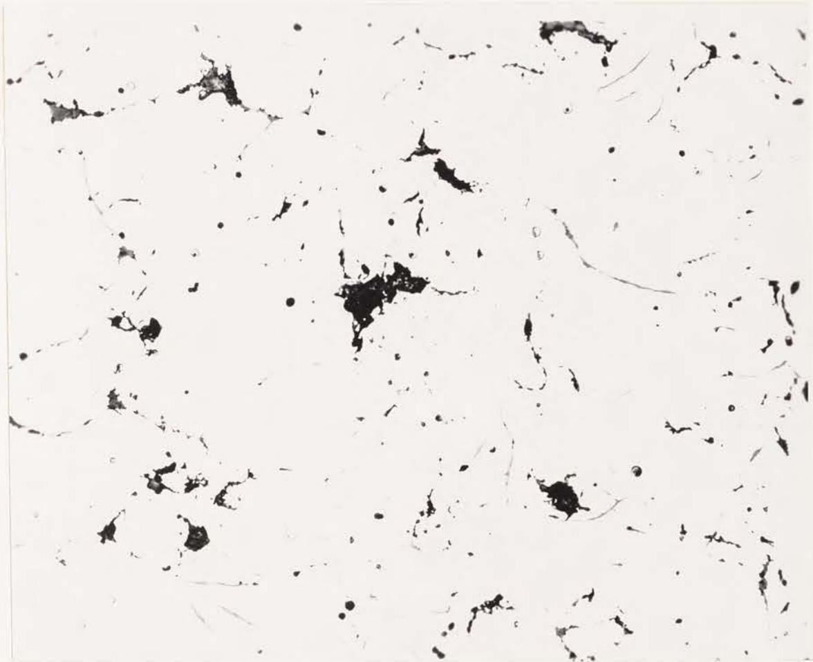
Figure 9: Fusion zone of a 1 percent silicon cast iron. Weld performed in a \text{SiO}_2 mold. Unetched 200X.
