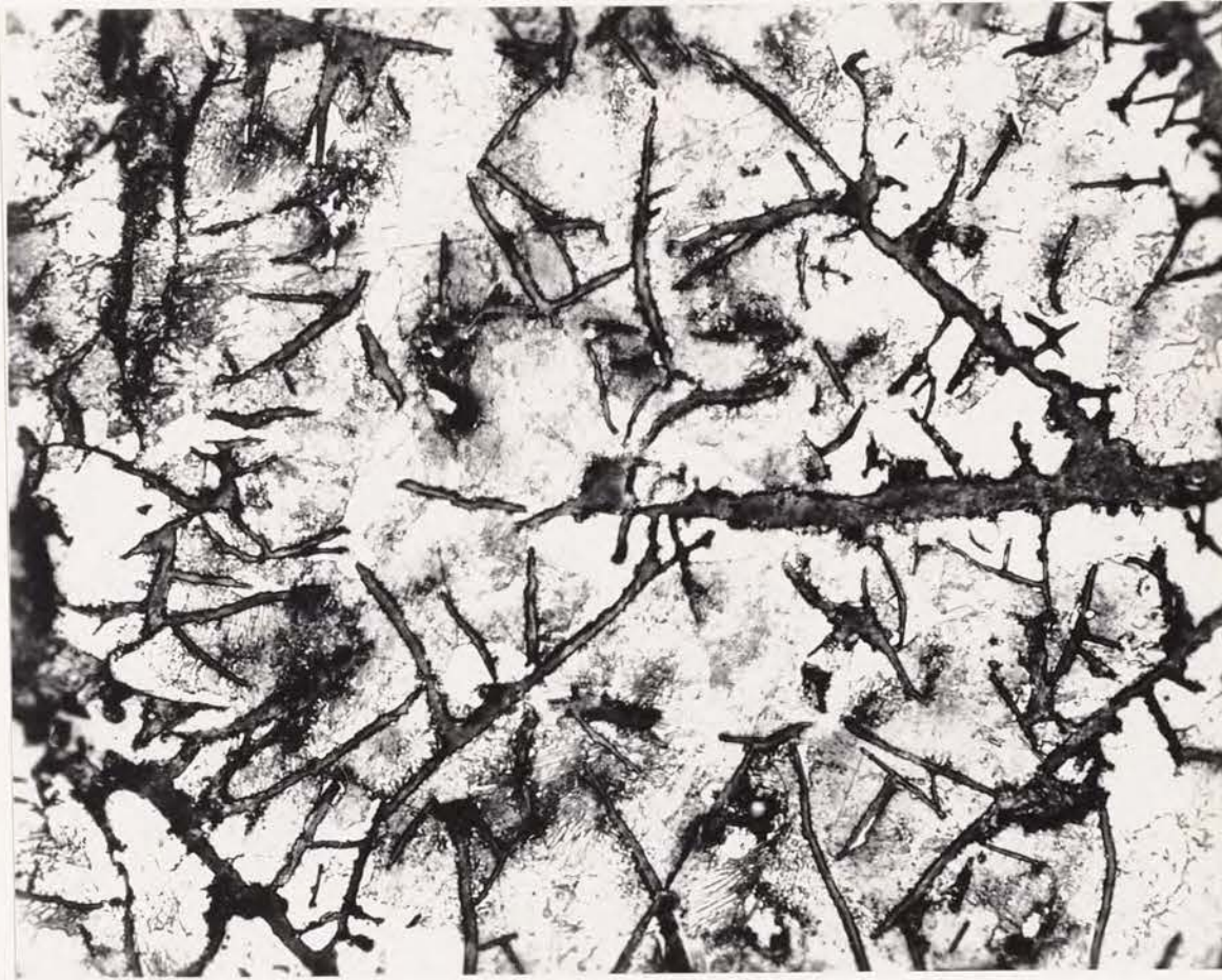
Figure 12: Fusion zone of a 2.7 percent silicon cast iron. Etched with 1 percent Nital, 500X.
