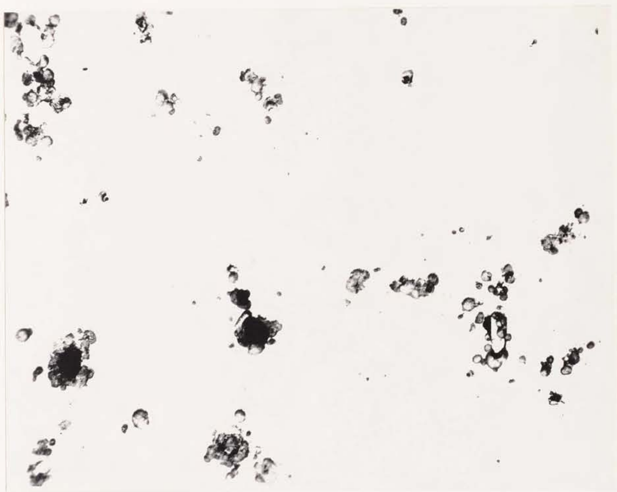
Figure 14: Nodular iron produced by the thermite process. Unetched 200X.
