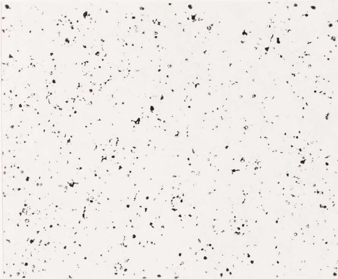
Figure 7: Edge of a typical fusion zone, unetched, 200X.
