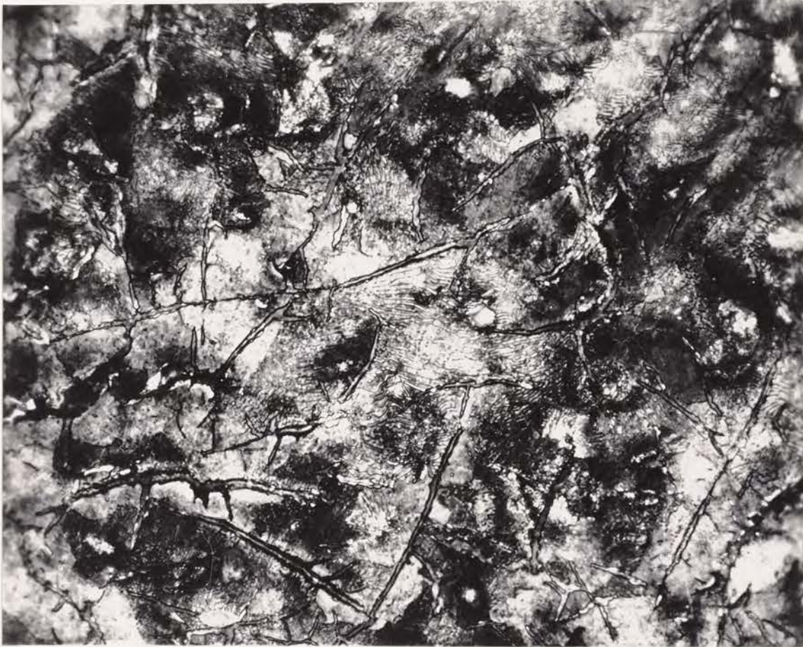
Figure 11: Fusion zone of 1 percent silicon cast iron. Etched with 1 percent Nital, 500X.
