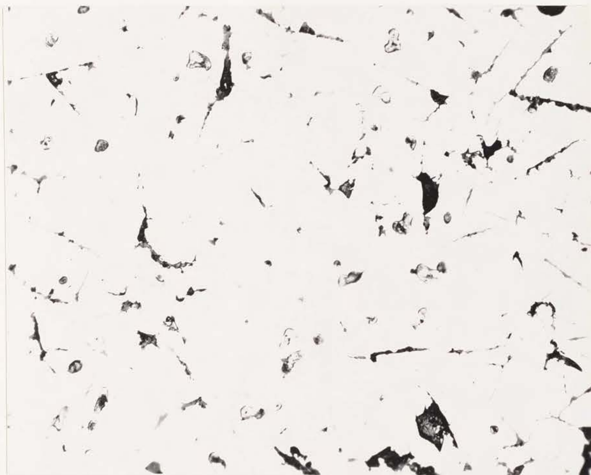
Figure 10: Fusion zone of a 2.7 percent silicon cast iron. Weld performed in an MgO mold. Unetched 200X.
