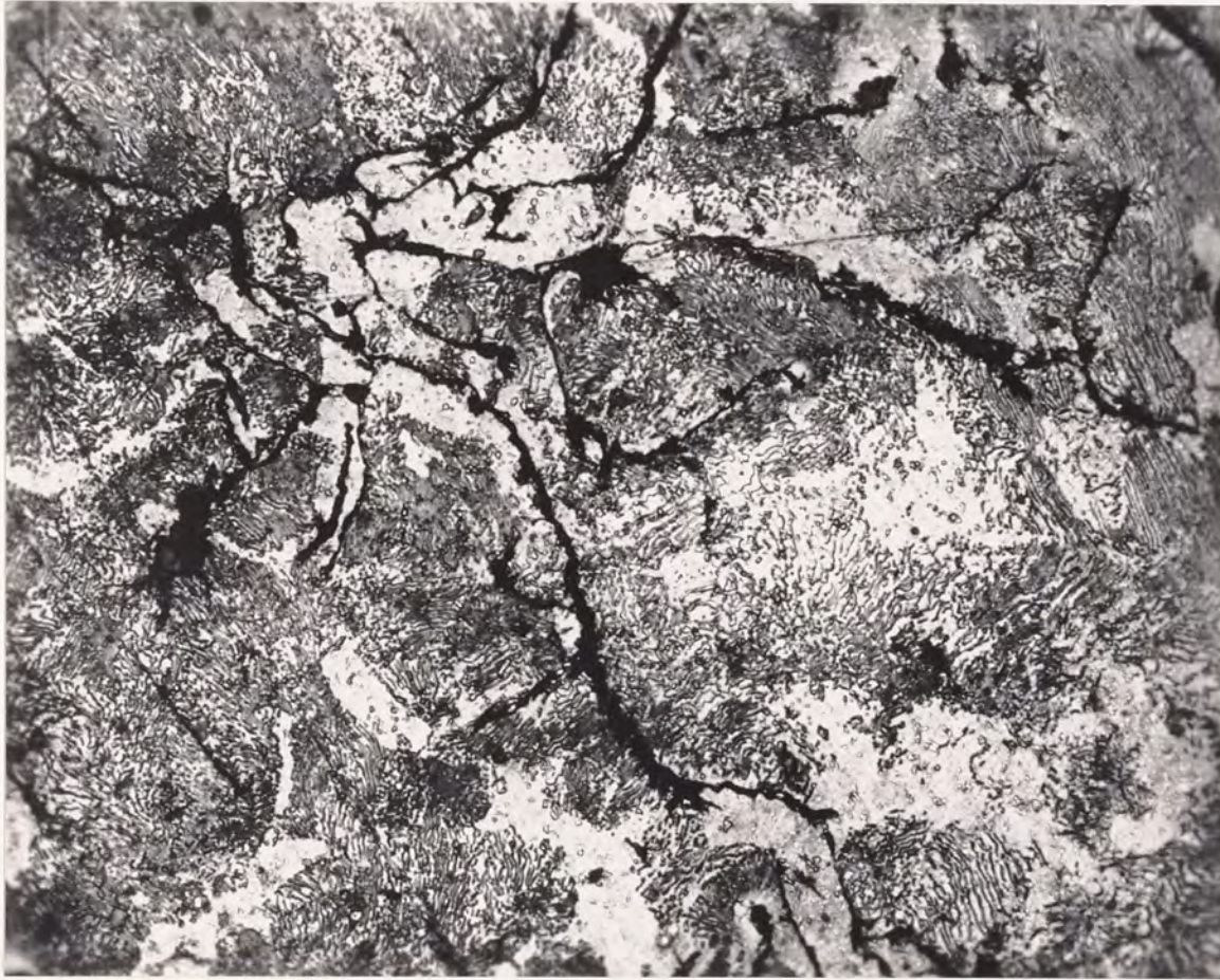
Figure 6: Heat affected zone of a typical weld plate, etched with 1 percent Nital, 500X.
