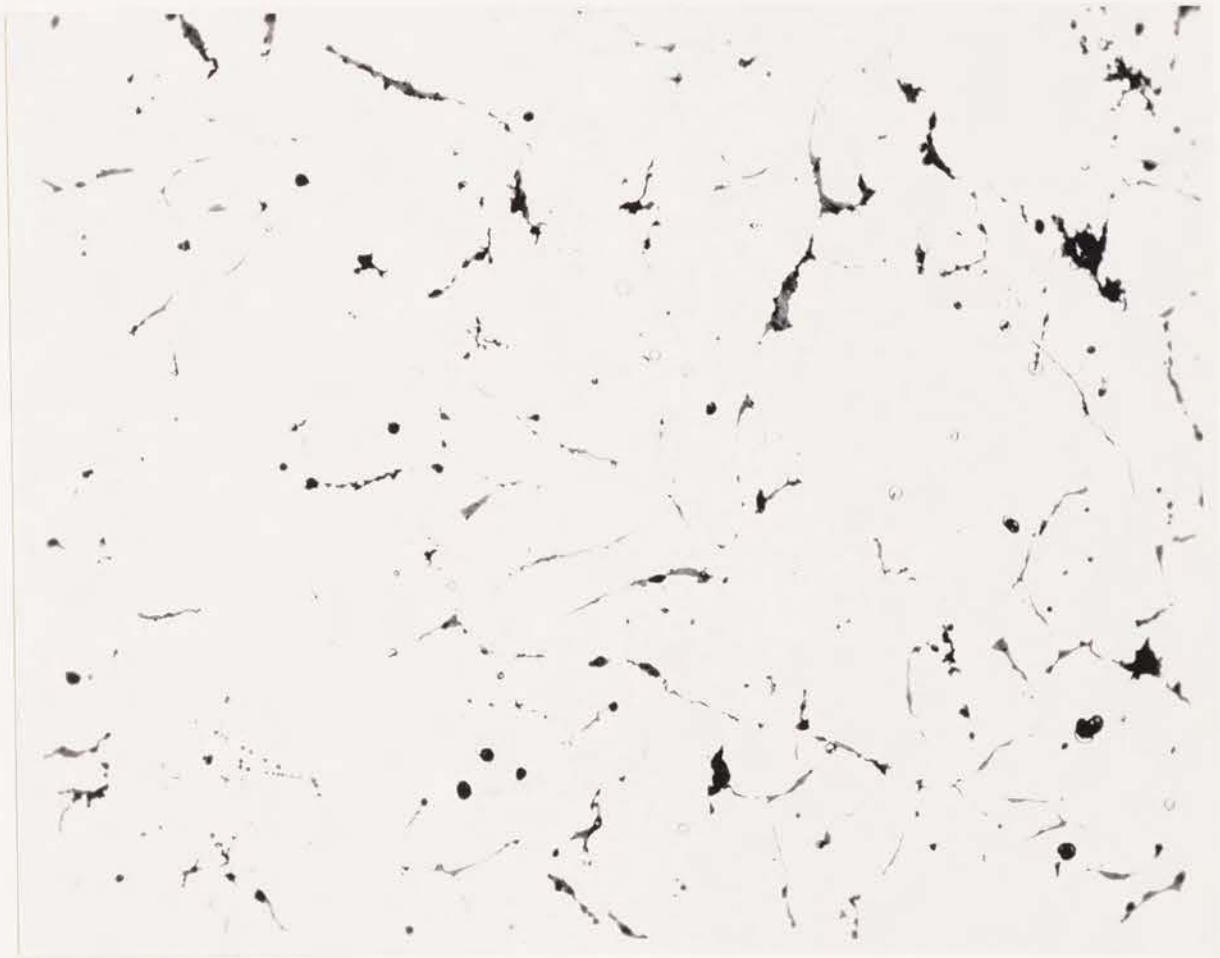
Figure 5: Heat affected zone of a typical weld plate, unetched, 200X.
