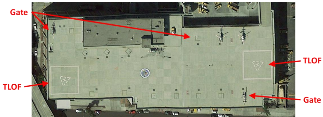
Fig. 16 Los Angeles Hooper Heliport displaying attributes of a “pier” topology. Map © 2018 Google.
