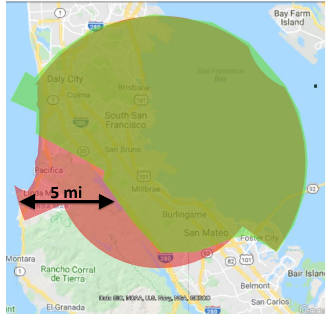
Fig. 38 Redesigned San Francisco class B airspace (green) compared to prior airspace (red) displaying reduction of controlled volume. Image © Google, 2019.
