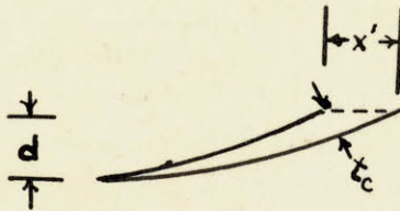
Figure 3 - ACTUAL GRINDING DEPTH OF CUT
