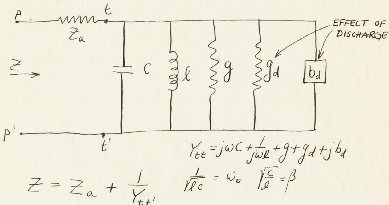
All impedances have been normalized to  $Z_0$ , the characteristic impedance of the circuit at  $PP'$ .
