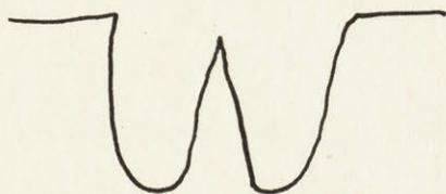
A calibrated echo box placed between slotted section and crystal produced a small pip on the trace by means of which frequency was measured.
