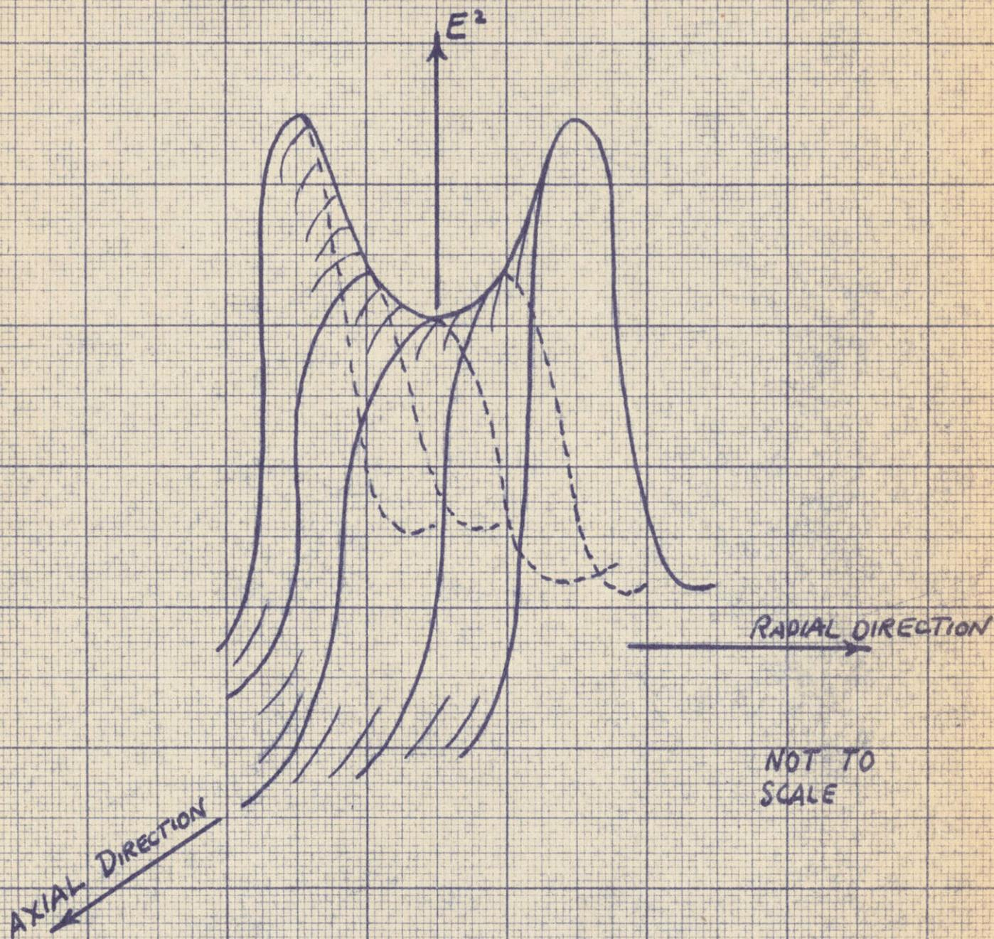
MICRO-WAVE ELECTRIC FIELD-STRENGTH IN DISCHARGE
