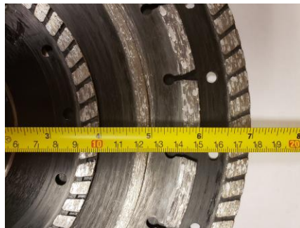
512 Figure 15: Different abrasive patterns on the different diameter blades.
