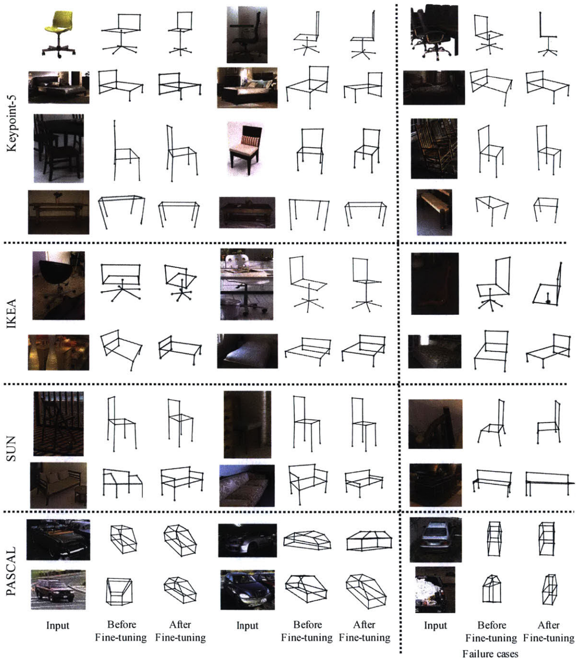
Figure 2-10: Qualitative results on Keypoint-5, IKEA, and SUN databases. For each example, the first one is the input image, the second one is the reconstruct 3D skeleton using the network before fine-tuning, and third one is using the network after fine-tuning. The last column shows failure cases.
