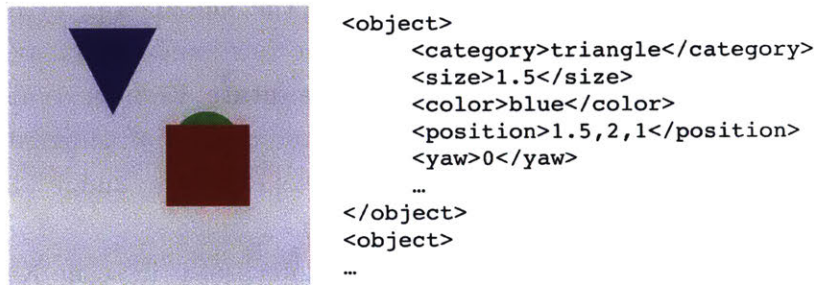
Figure 4-3: An image and part of its scene XML , encoding the background and the category, appearance, position, and pose of objects in the image.
