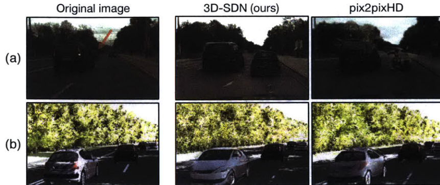
Figure 4-11: Comparing 3D-SDN (ours) and pix2pixHD [Wang et al., 2018c]. (a) We successfully recover the mask of an occluded car and move it closer to the camera while pix2pixHD fails. (b) We rotate the car from back to front. With the texture code encoded from the back view and a frontal pose, our model can remove the tail lights, while pix2pixHD cannot, given the same instance map.
